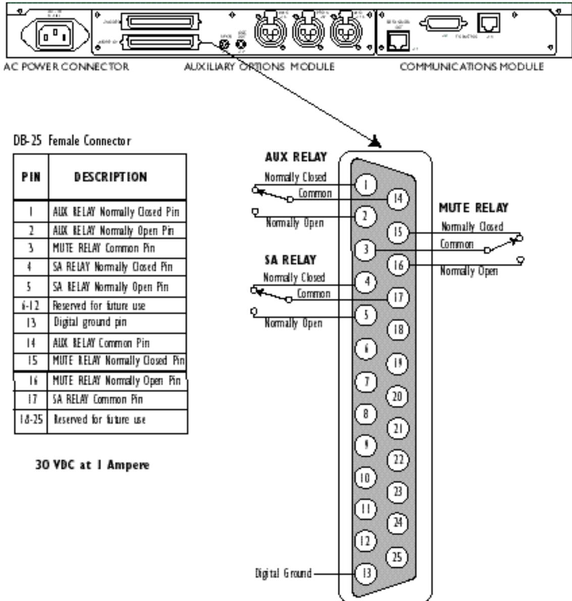
Figure 9-4 Relay Outputs Connector (J3) Pinout Diagram
