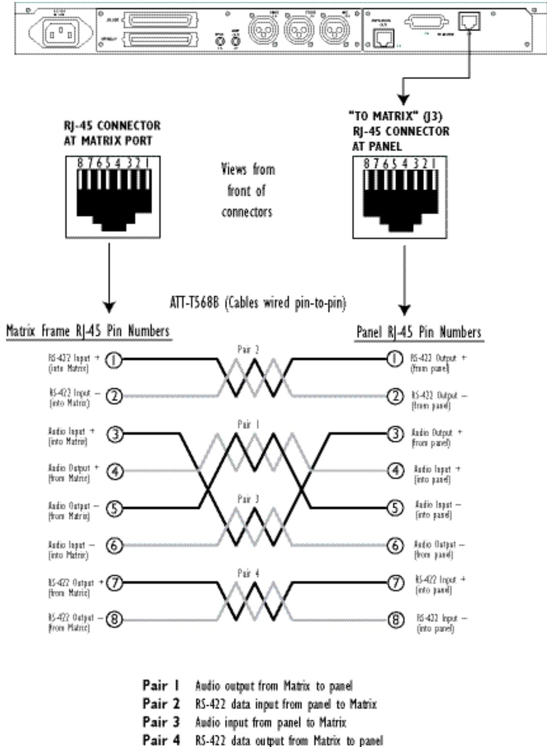
Figure 9-2 RJ-45 to Matrix Connector Pinout Diagram
