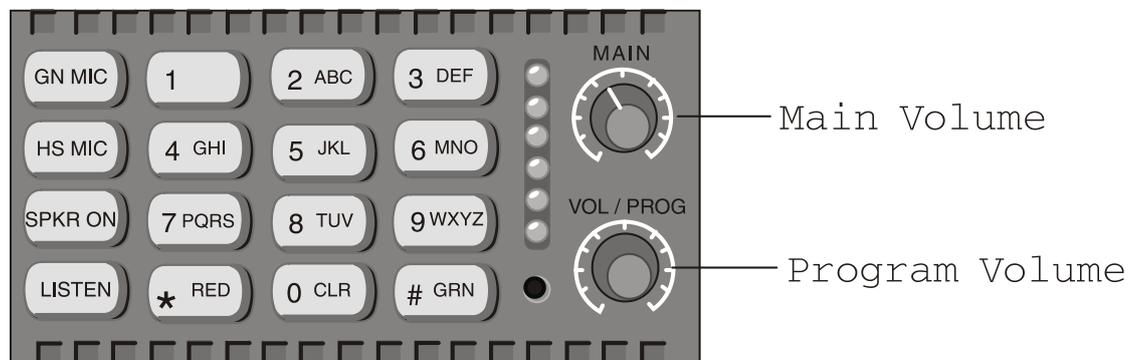
Figure 4-3: Main volume and program input volume controls
