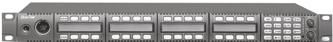
Figure 3-5 I-1430E 32 key I-Station Display with keypad
