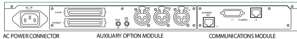
**Figure 7-1 Rear Panel of an i-Series Intercom Panel**
