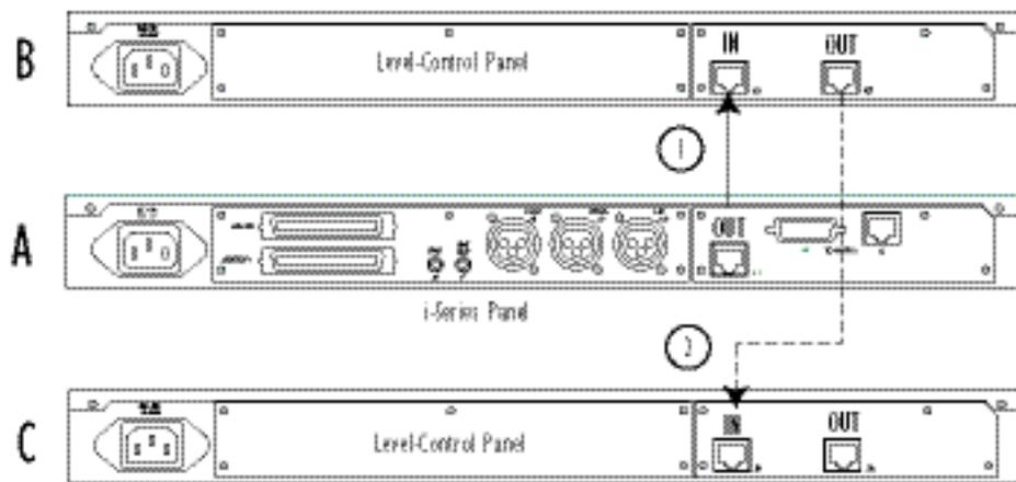
1. Connect the OUT connector of the main i-Series panel (A) to the IN connector of the first v-station expansion panel (B).
