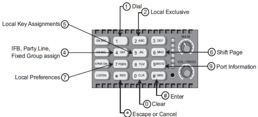
Figure 6-1: Advanced features, accessed from the numeric keypad
