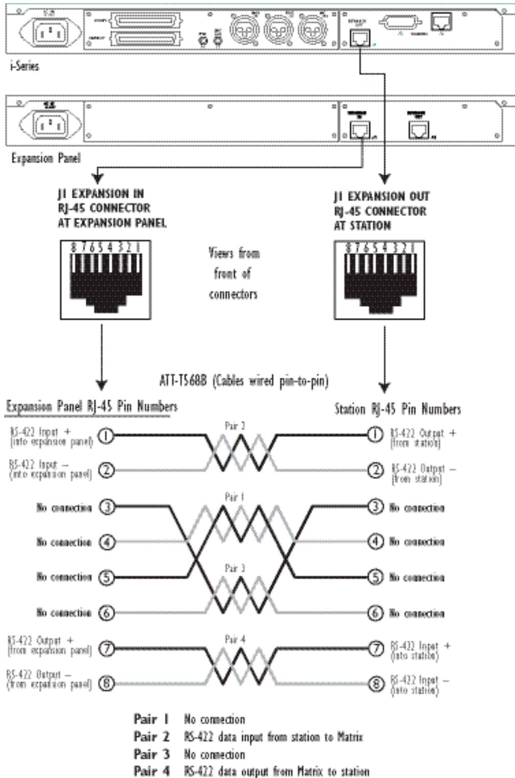
Figure 9-1 Expansion Out Connector Pinout Diagram
