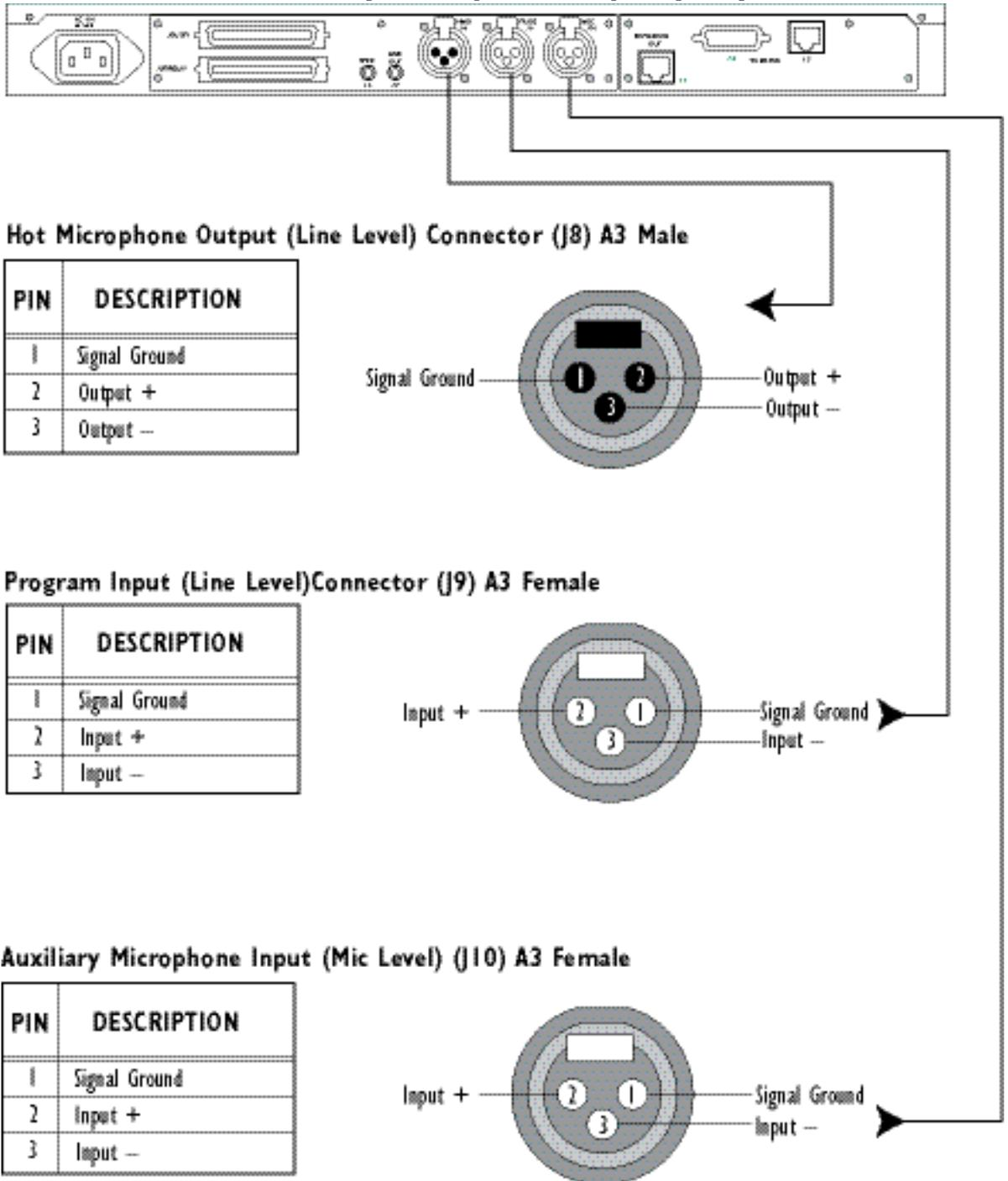
**Figure 9-6 Connector Pinout Diagrams for Hot Microphone Output (J8), Program Input (J9), and Auxiliary Microphone Input (J10)**
