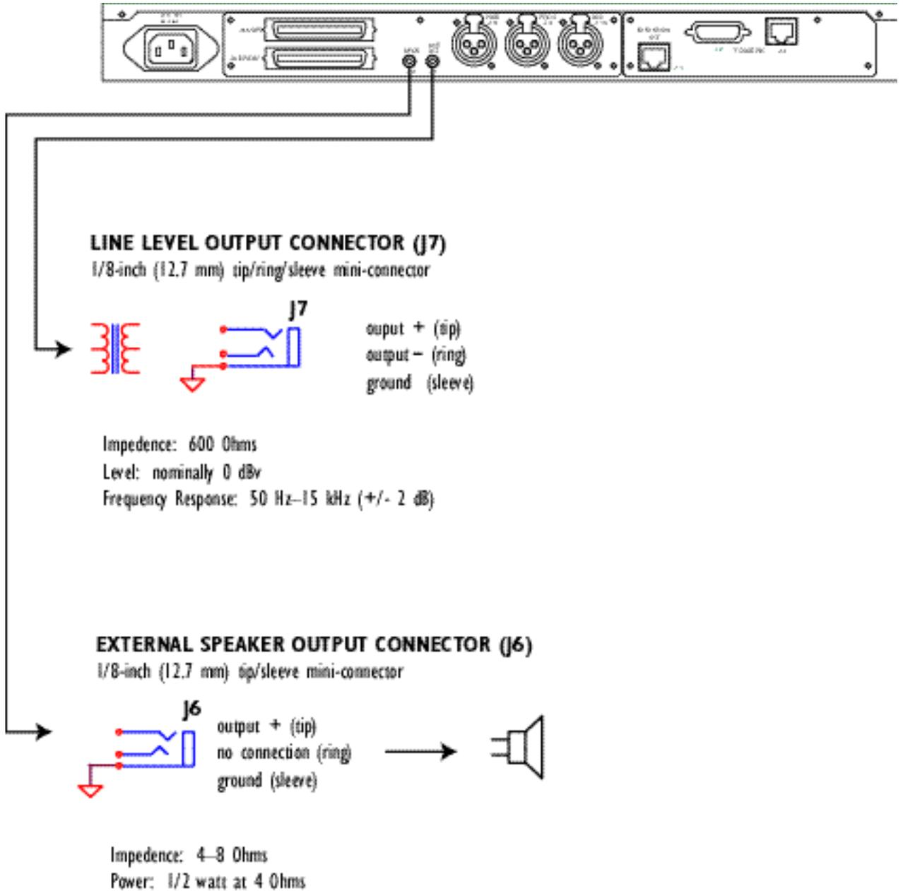
Figure 9-5 Connector Pinout Diagrams for Speaker-Feed Output and Line-Level Output
