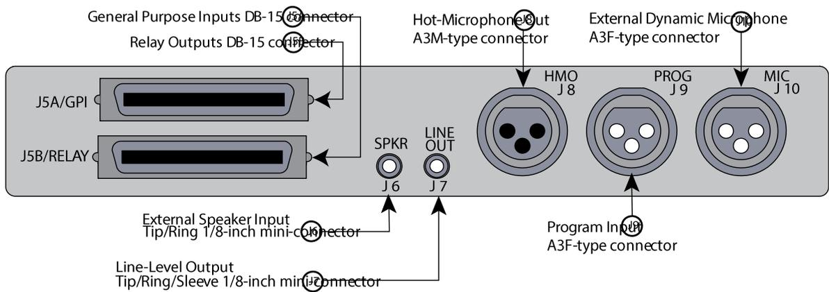
Figure 7-3 Auxiliary Options Module Connectors
