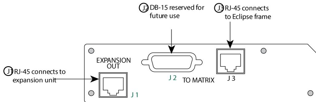
Figure 7-2 Communications Module Connectors
