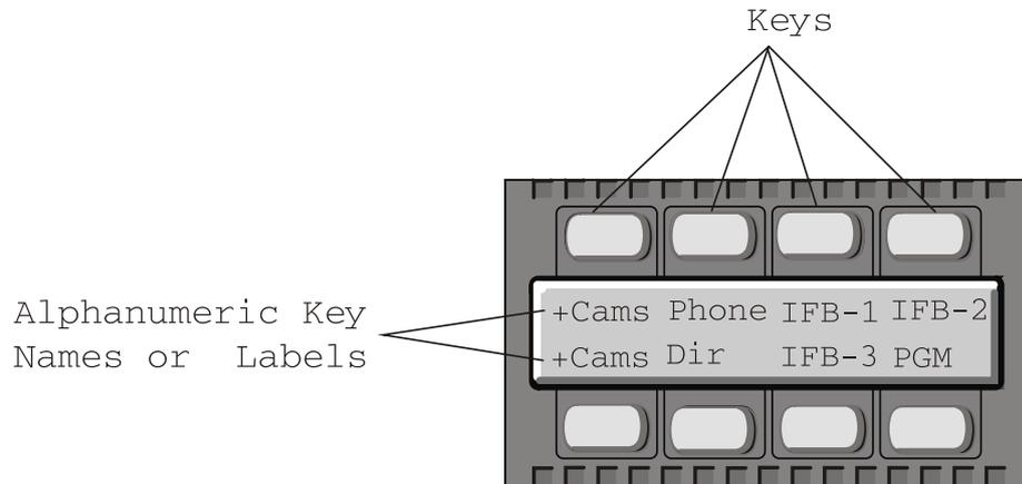
**Figure 2-1: Labels on a key module**
