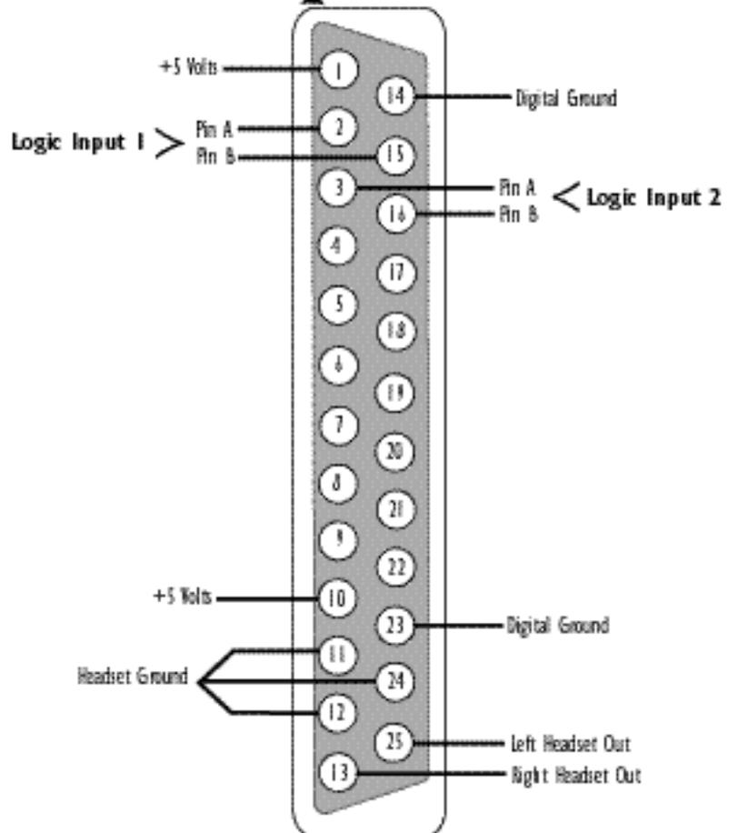
Figure 9-3 General Purpose Inputs Connector Pinout Diagram
