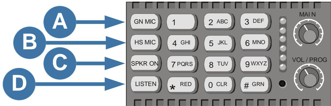
Figure 5-1: Four basic function keys, function module
