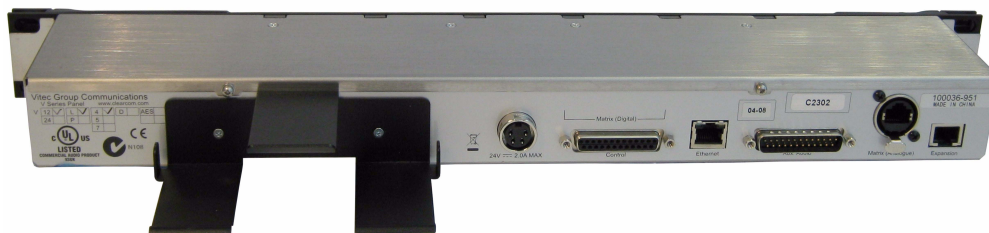
Figure 4: V-Series Rack Mount Panel with PSU Removed
