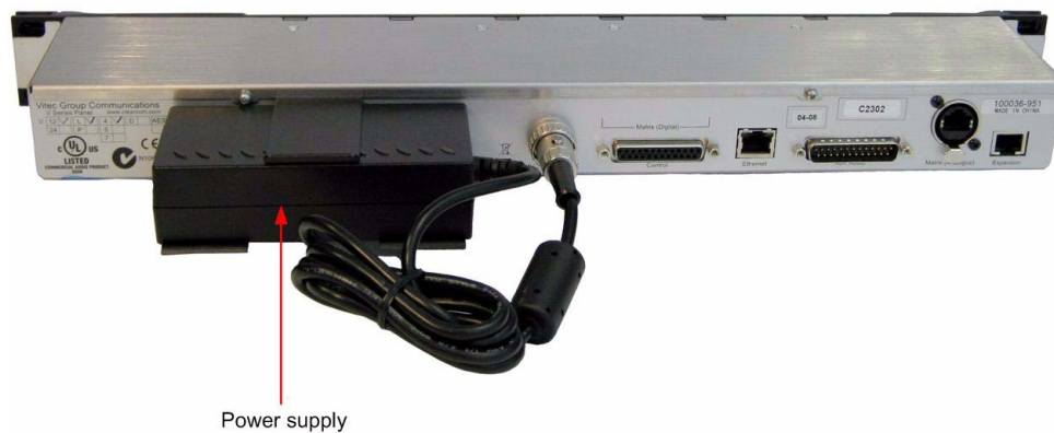
Figure 3: Power Supply in Cradle on Rack Mount Panel
