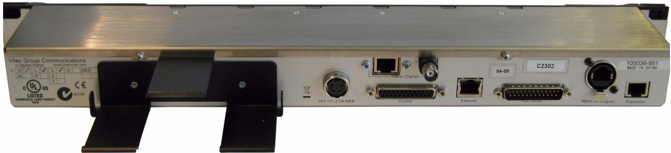
Figure 11: Rack Mount Panel Upgrade with Lid Replaced
