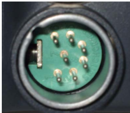
Figure 16: Front View of XLR-7M Headset Connector Assembly Fitted
