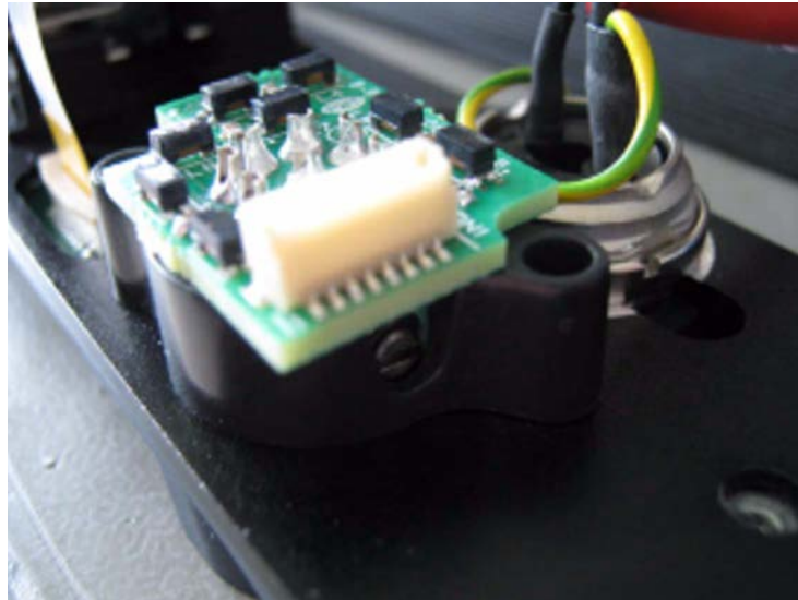
Figure 12: Fit the XLR-7M Headset Connector Assembly
