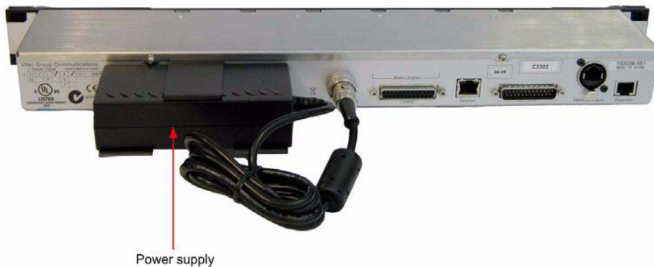
Figure 1: Power Supply in Cradle on Rack Mount Panel
