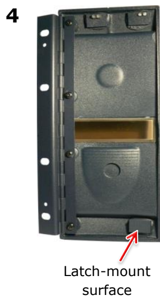
Figure 2-4: Latch-mount surface, inside the Eclipse HX door
