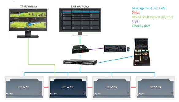
On an LSM-VIA MultiReview setup, the XClient-VIA receive the proxy streams multicasted from the XT-VIA servers, and XS-VIA network servers, and routed to the Control Network (PC LAN) through the switch. See section "Setting Up the LSM-VIA MultiReview Environment" on page 8 for a detailed description.
