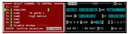
Use the ↑/↓ arrow keys to select the channel and press **ENTER**, or directly press **ALT**+the number of the channel as highlighted in green. The Play channels already assigned appear in grey and cannot be selected. Select "0 – Disable Window" if you don't want to assign any channel to the window. Depending whether a Play or Record channel is assigned to the VDR Panel window, its content is automatically updated.
