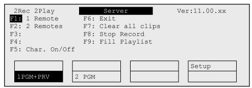
The Main menu has special function key operations as shown above, as well as the "soft" keys options to enter 1PGM+PRV, 1PGM, or 2PGM modes (if available) and to enter the **Setup** menu to configure your remote controller or to add special functions to your application.
