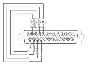
The relay must be connected between the ground and the corresponding TTL input on the DB-25.
