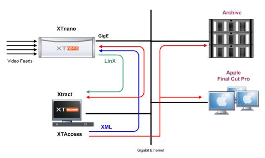
XT Access is directly connected to the XTnano servers through the Gigabit network. It runs on an XP workstation and is controlled, in this context, by Xtract via XML files.
