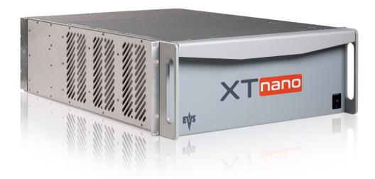
The EVS XTnano servers are full digital in PAL (625i), NTSC (525i), 720p, and 1080i standards. These multi-channel, disk-based video servers are ideal for a wide range of broadcast applications, from sports and live production to playout and transmission.
