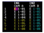
You will allocate the source audio mono channels as shown above when you want to send the audio mono channels from REC1 to all other record channels.
