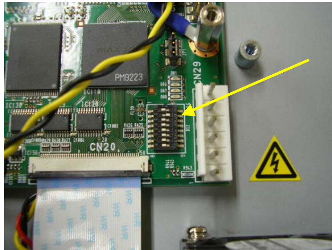
Fig. 10 Set DIP switch DS2-2 to ON
