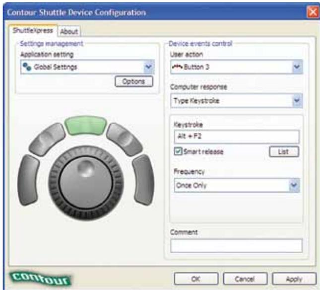
Figure 139. Configuring ShuttleXpress button 3 to actuate the GLM Setup Load function.
