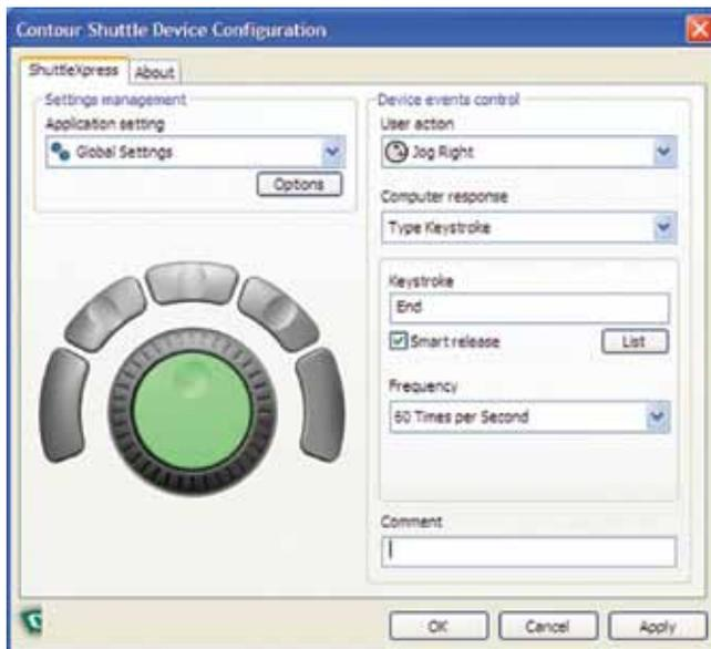
Figure 143. Configuring ShuttleXpress Jog knob to actuate the basic GLM Level Up function when rotated right (Jog Right).
