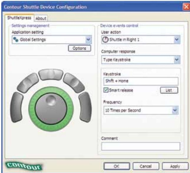
Figure 146. Configuring ShuttleXpress Shuttle ring to actuate faster GLM Level Up function when rotated right.
