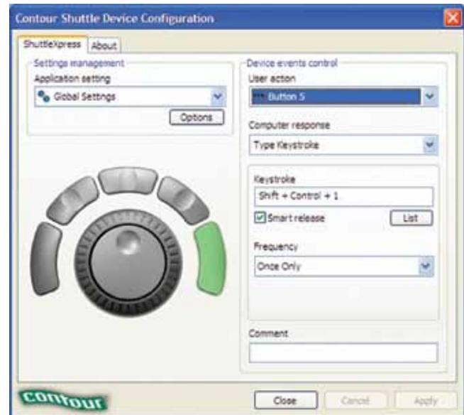
Figure 141. Configuring ShuttleXpress button 5 to actuate the GLM Preset Level 1 function.
