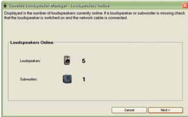
Figure 15. System Setup Wizard Loudspeakers Online counter screen
