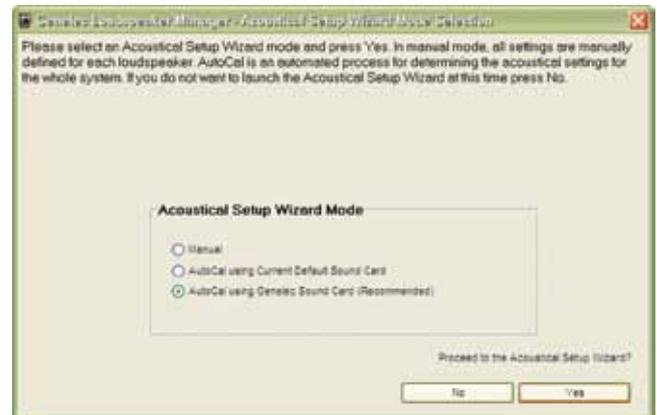
Figure 49. Acoustical Setup Wizard Mode default setting for Network Interface Device with sound card
