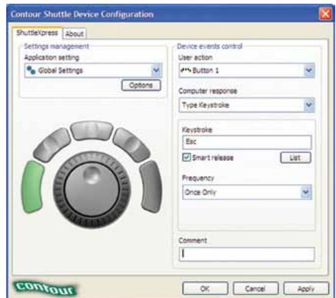
Figure 137. Configuring ShuttleXpress button 1 to actuate the GLM Mute function.
