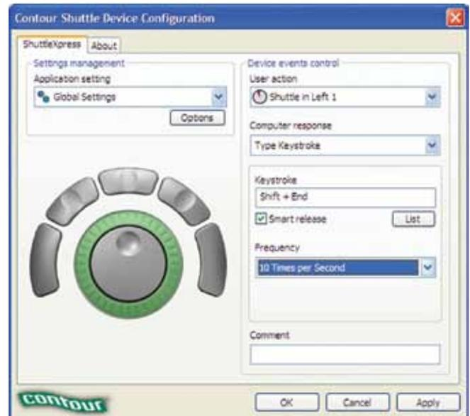
Figure 144. Configuring ShuttleXpress Shuttle ring to actuate faster GLM Level Down function when rotated left.
