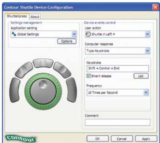
Figure 145. Configuring ShuttleXpress Shuttle ring to actuate very fast GLM Level Down function when rotated further left.
