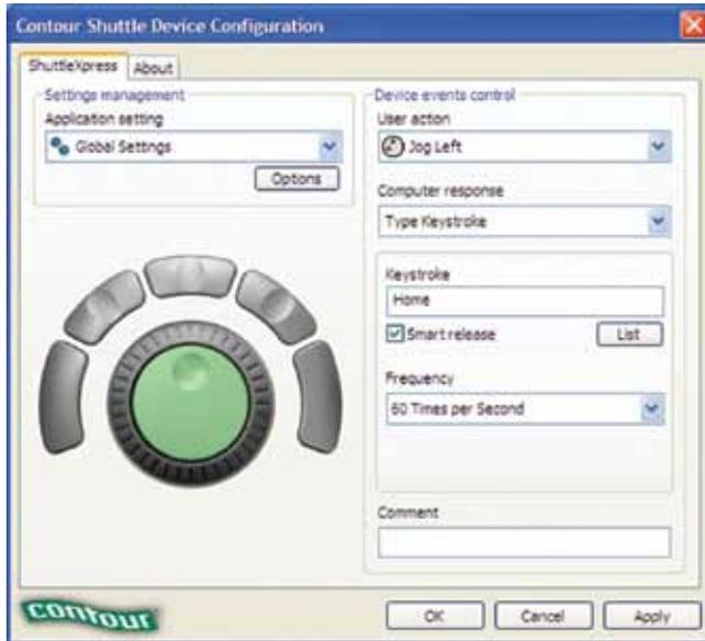
Figure 142. Configuring ShuttleXpress Jog wheel to actuate the basic GLM Level Down function when rotated left (Jog Left).
