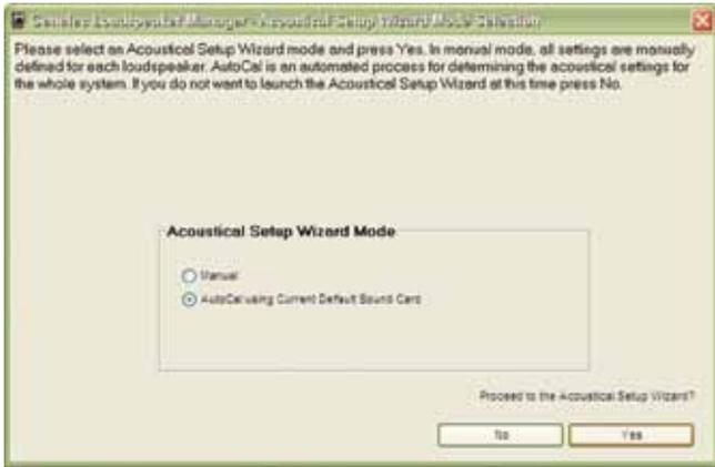
Figure 50. Acoustical Setup Wizard Mode default setting for Network Interface Device without sound card
