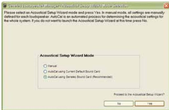
Figure 57. Starting AutoCal in the Acoustical Wizard Mode Selection window
