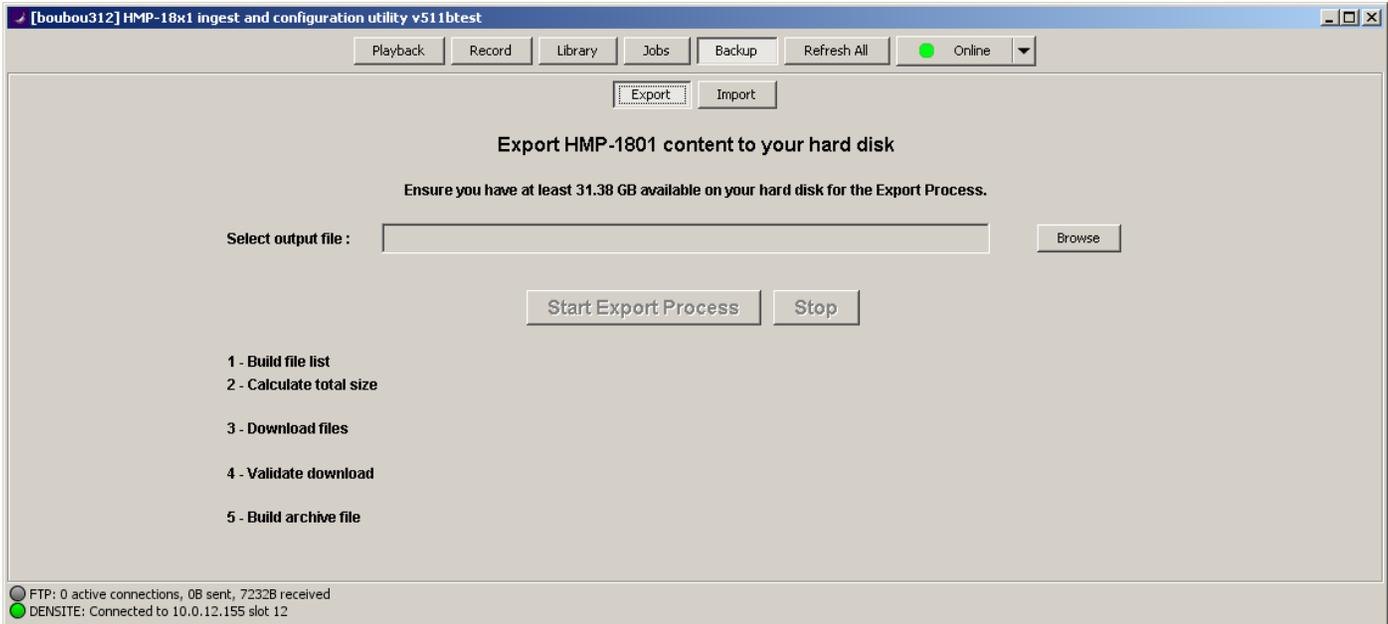
To save the contents of the HMP-1801 Compact Flash to an external storage medium:
