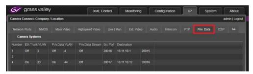
C2IP tab with overview of C2IP IP and VLAN settings. Note:
