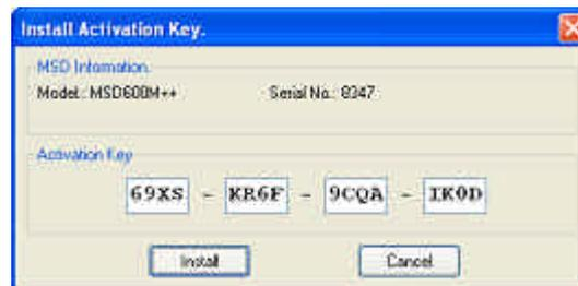
When opening the window 'Install Activation Key' DK-Matrix will disconnect from the MSD if it is in ON-Line mode. After a few seconds the Activation Window will show the MSD-Type, Serial Number and the current Activation Key installed in the MSD.
