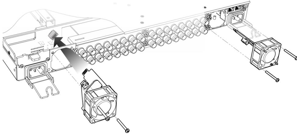
The two ventilator fans are mounted at different angles, as shown in the above figure.
