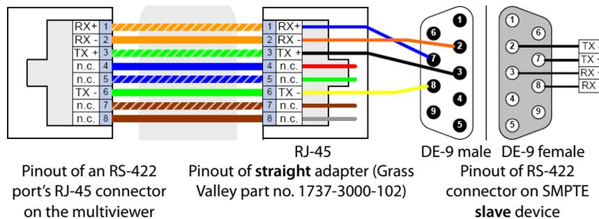
*Standard wiring between multiviewer and devices wired to SMPTE "slave" specification (e.g. most routers, Ross Synergy switchers, Neveon ETH-CON)*
