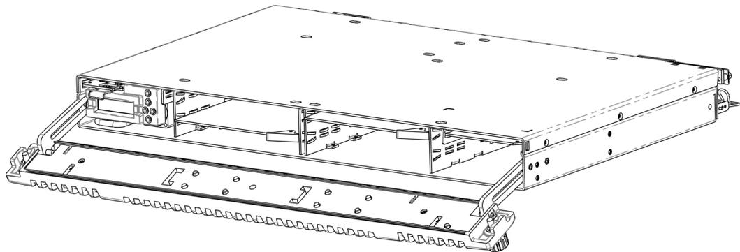
The front door of the Kaleido-MX (1RU) frame is fastened in place by two captive thumbscrews, one at each end of the door.
