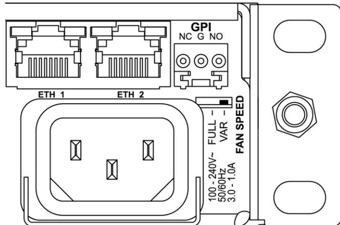
Use a small tool (e.g., a pen tip or a small screwdriver) to change the switch setting.
