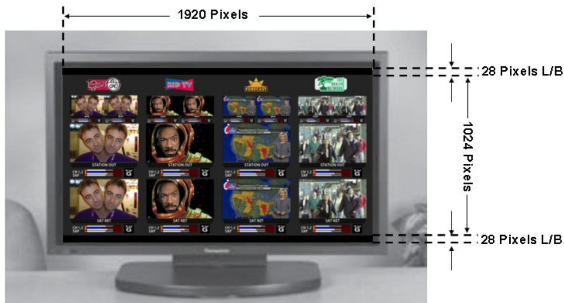
Figure A1: Kaleido-Quad-Dual output on a 1920x1080 display showing black bars top and bottom
