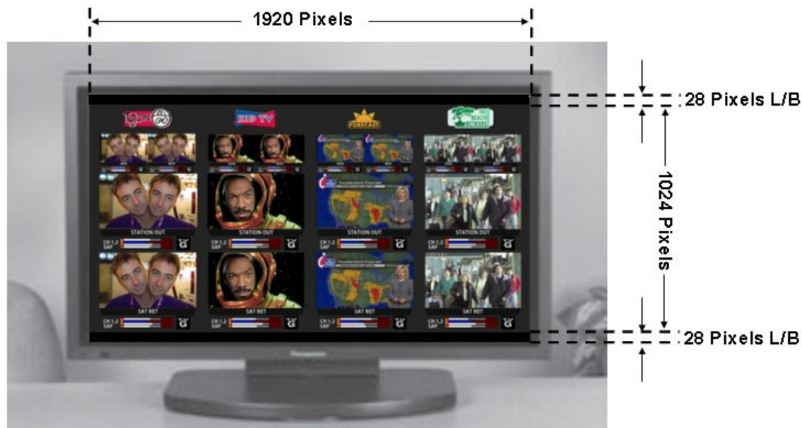
Figure A1 Kaleido-Alto output on a 1920x1080 display showing black bars at the top and bottom
