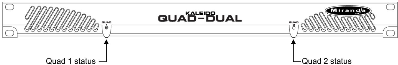
Figure 3.1 Front panel Status LEDs
