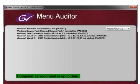
2 Select **Scan**. The Auditor will check each relevant installation and indicate the state of the computer environment.
