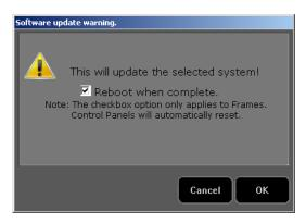
If the Reboot when complete box is checked, the Video Processor Frame, optional Image Store, and all associated Control Panels will reboot after the **OK** button in the Software update warning dialog is selected. If the box is not checked, you will need to manually reboot the Video Processor Frame and optional Image Store hardware after the software files have finished installing. Control Panels are always rebooted after a software update.
