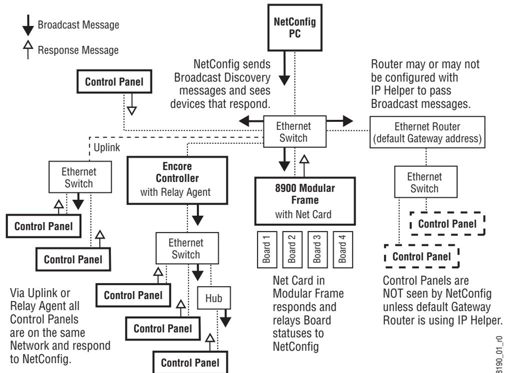
**Note** We generally recommend using unmanaged switches, instead of hubs, on networks. A hub may be used with a single device to extend beyond the Ethernet 100 meter limit. We do not recommend attaching multiple devices to a hub since this commonly introduces Ethernet message collisions that can affect overall system performance.
