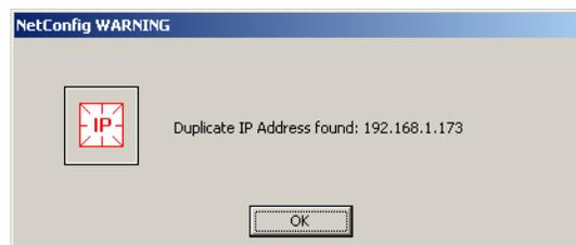
To resolve the duplicate IP address, go to the Set IP window, ensure All Devices is selected, and sort the list by IP Address. The devices with duplicate IPs will be listed together. Choose one to change, and give it a unique IP address, using the standard IP address configuration procedure described earlier.
