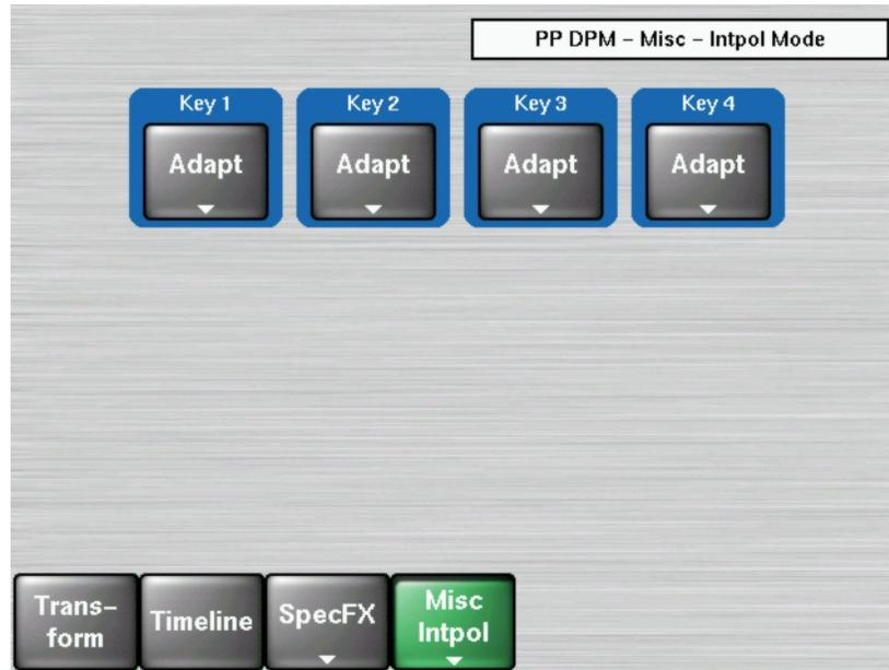
**Frame Interpolation Mode** button (See [Figure 17](#))—**Frame Mode** preserves fine lines in source material. Kayak interpolates pixels to Field Mode when there are fine horizontal lines in the source material. Some fine lines may be lost for example in text or characters when in motion. Using **Frame Mode** preserves the text and characters.
