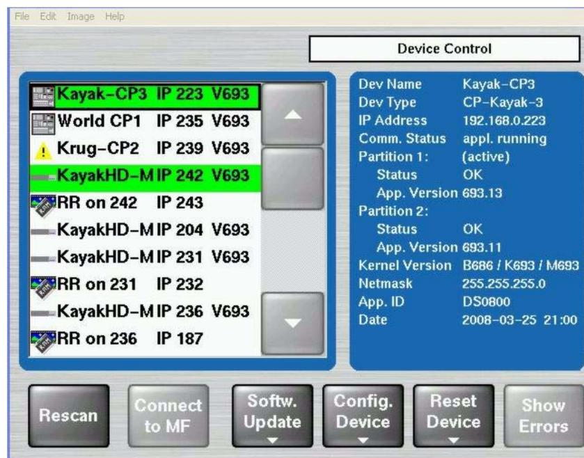
7. Select the device for software installation from the scrolling list in the **Device Control** menu.
