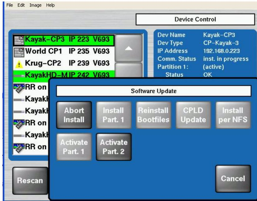
**CAUTION** Use only the **Abort Install** button to cancel installation. Do not interrupt the installation using any other method.
