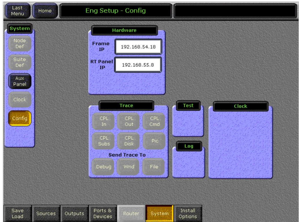
Also, if possible record the Windows 2000 TCP/IP address using the standard Windows 2000 interface. You may use the Touch Screen to access the Windows settings but you will need to use a mouse and keyboard connected to the Menu panel for entering or changing the IP address values. To record the current Menu panel address do the following.
