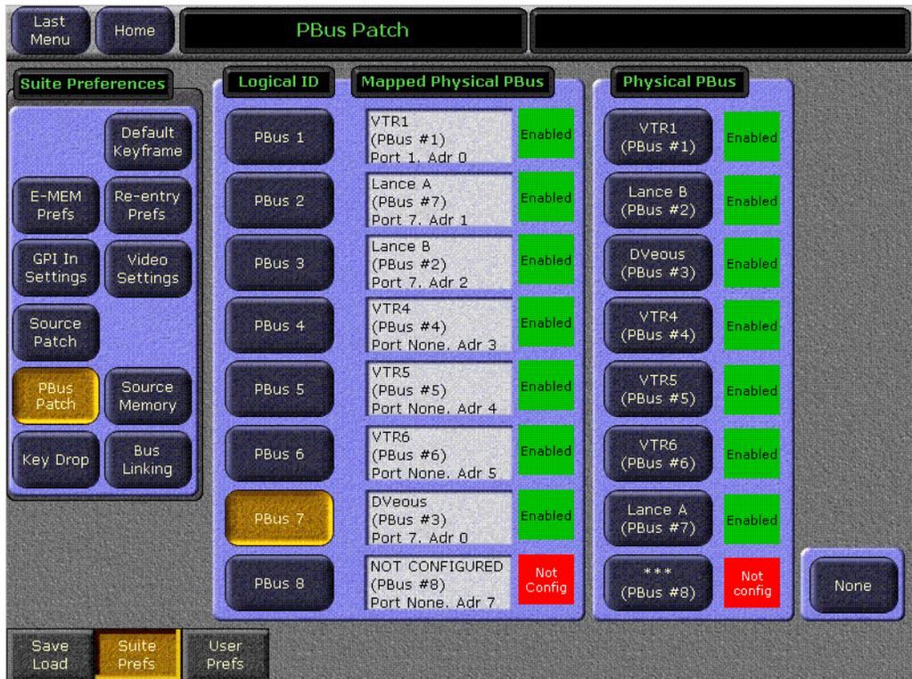
To patch the PBus devices, select a Logical ID of the device in the left pane, and then select the Physical PBus button on the right pane. The current mappings are reported in the central status boxes.
