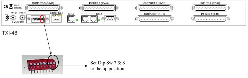
The TXI-48 is shipped from the factory to work serially. To make the TXI-48 work using Ethernet.
