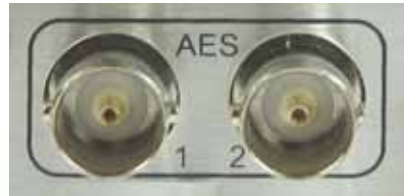
Standard coaxial/unbalanced output audio connectors
