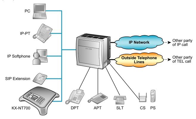
The following features are available when the unit is used as a SIP extension. Refer to the PBX documentation for details.
