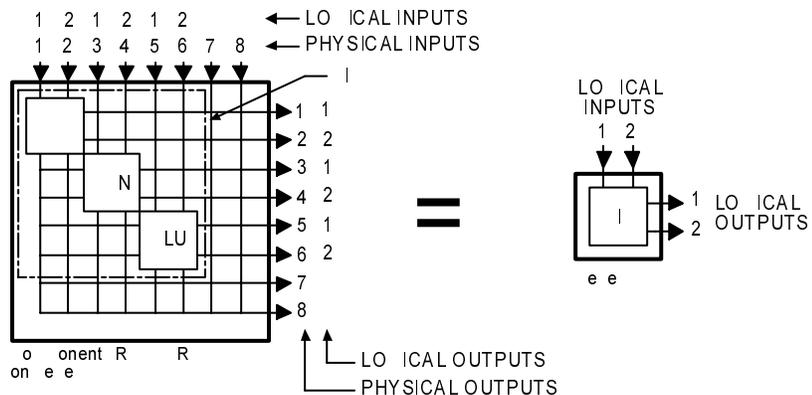
As a general rule, users control the switching of levels, but component switching is handled automatically by the switching system. In the example above, a user could specify a single logical switch, such as VID Input 1 to VID Output 2. This would result in Win3500 taking three physical switches by activating crosspoints (1,2), (3,4) and (5,6).
