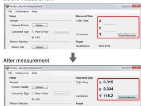
During measurement, the measured values will be updated every time data is received from the probe. Therefore, the measurement intervals depend on the performance of the probe.
