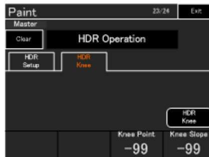
The screenshot shows the 'Paint' menu with an 'HDR Operation' sub-menu. The menu includes a 'Clear' button and two buttons: 'HDR Setup' and 'HDR Knee'. Below the menu, a table displays the following values:
