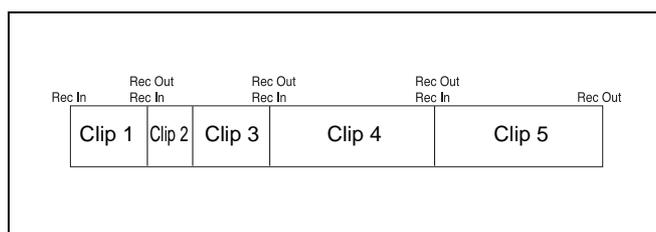
This unit can also fast forward in clip units (clip jump). This allows you to quickly jump to a position close to the target frame by jumping to the start or end point of one clip after another.
