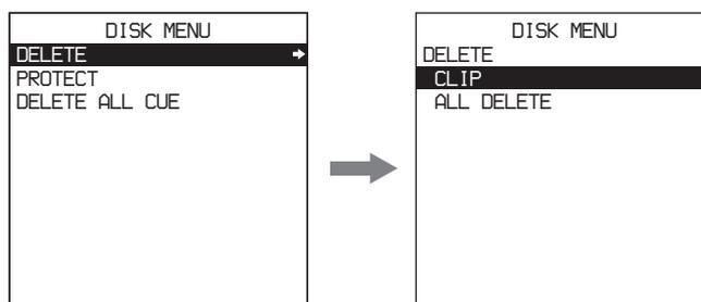
To display the delete operation menu, select DELETE in the Disk menu and press the  $\Rightarrow$  (OUT) button. In the delete operation menu, select CLIP or ALL DELETE and press the SET button to delete individual clips or all clips.
