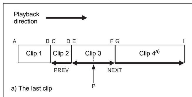
When you press the PREV button or the NEXT button at the current position (point P), the unit behaves as follows.
