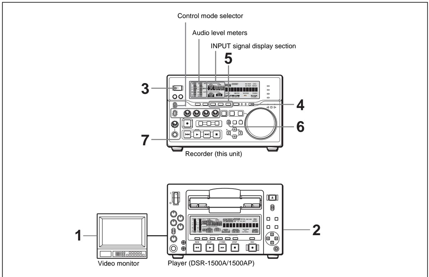
When controlling this unit from an editing control unit connected to the REMOTE IN (R)connector, see “Control mode selector” on page 15 and the description of the REMOTE I/F menu item on page 72.
