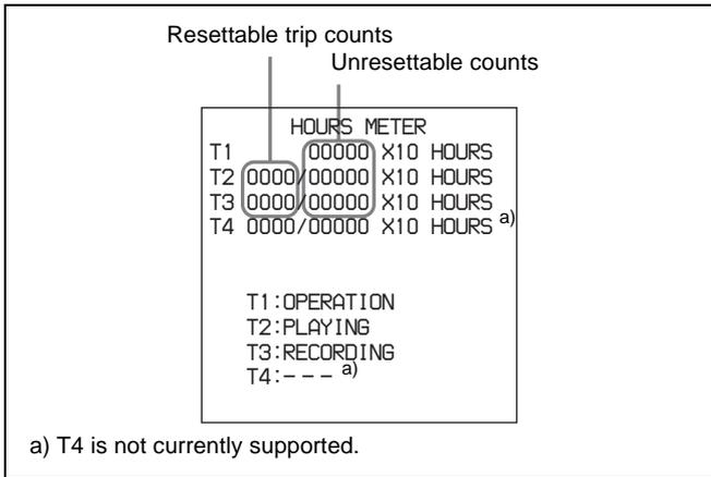
The four-digit value to the left of the slash (/) is the resettable trip count, and the right value is the cumulative total from manufacture.
