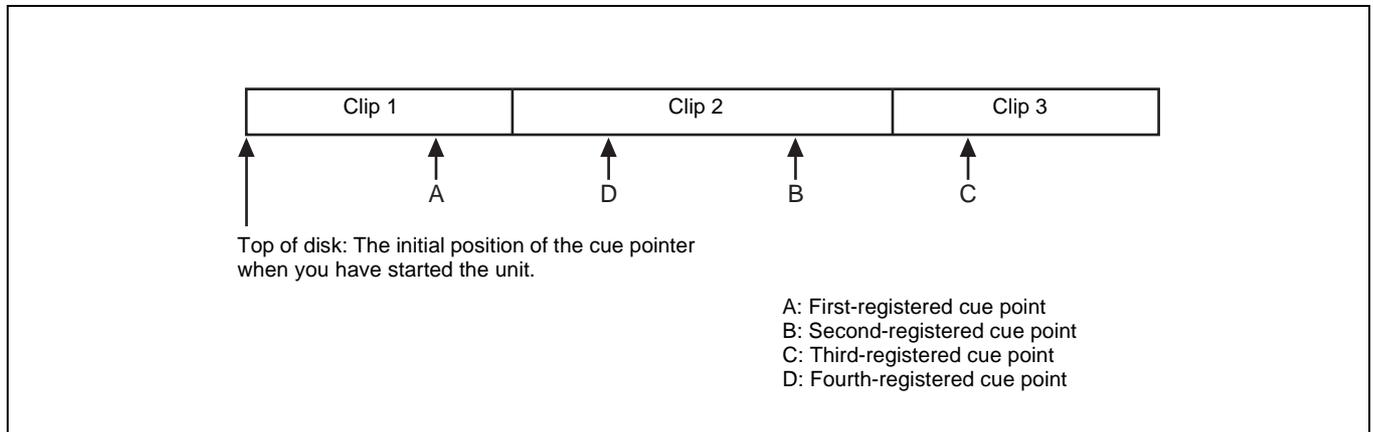
If cue points are registered as shown in the above figure, pressing the NEXT button repeatedly with the  $\hat{\uparrow}$  (CUE) button held down makes the cue pointer jump in the order ARBRCD.
