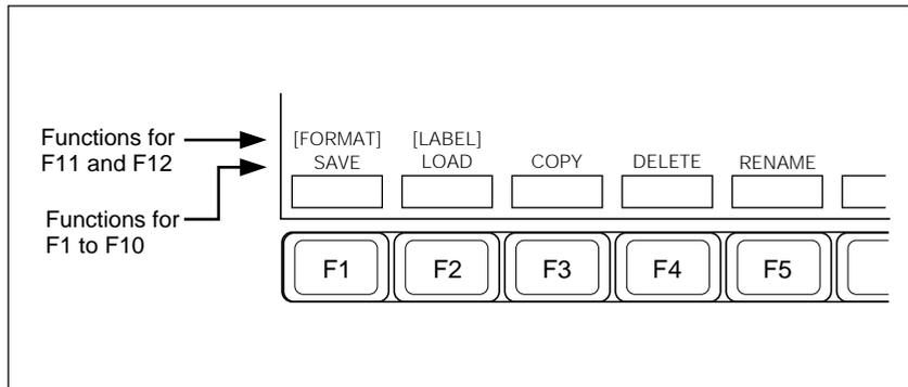
To select the upper row of functions (indicated as F11 to F20), hold down the SHIFT button to interchange the two rows of indications, then press the corresponding function key F1 to F10.
