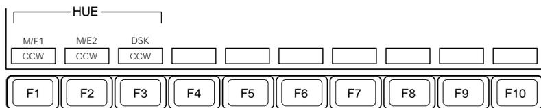
**5** Press one of F1 (M/E1) to F3 (DSK) to select the HUE path type for the corresponding bank.
