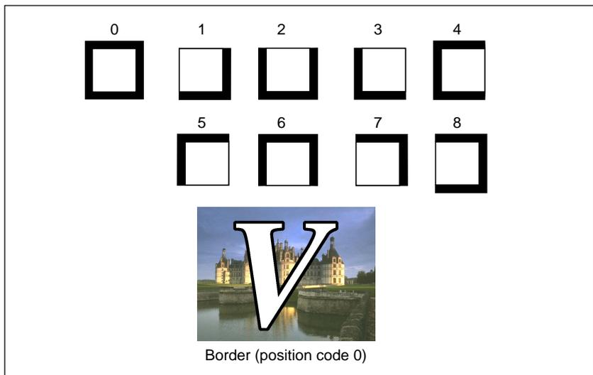
**Drop border or shadow:** When using the BKDS-7270, there are eight positions (numbered 1 to 8) to apply a drop border or shadow. When using the BKDS-7271, you can adjust the drop border or shadow position continuously through the eight positions.
