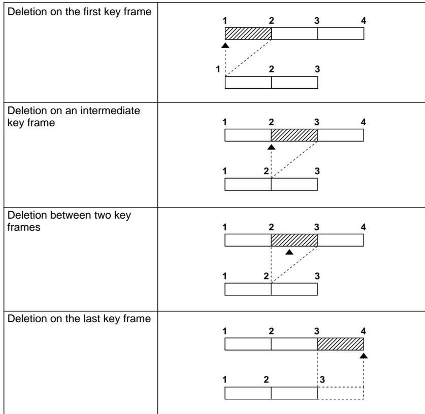
Key frame deletion position and changes in effect duration
