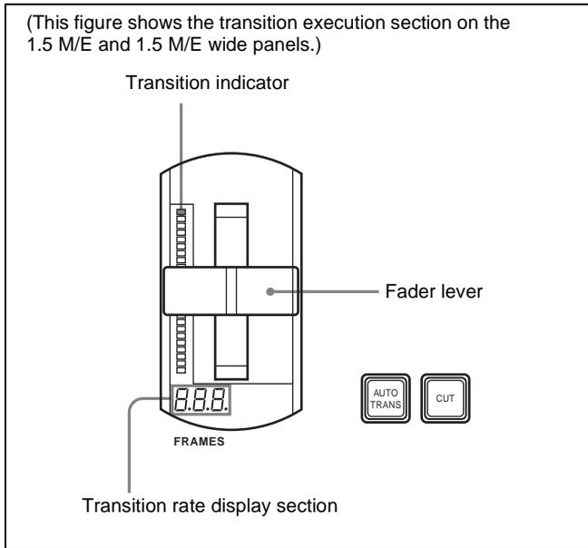
**Fader lever:** Move the lever up and down to execute the transition.
