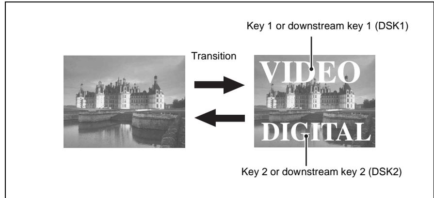
A linear key is a type of luminance key, but with less variation in gain, allowing more precise adjustment.
