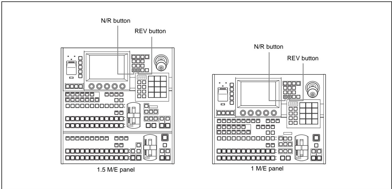
**To select the normal direction:** Turn both the [REV] button and [N/R] button off, so that they are not lit.
