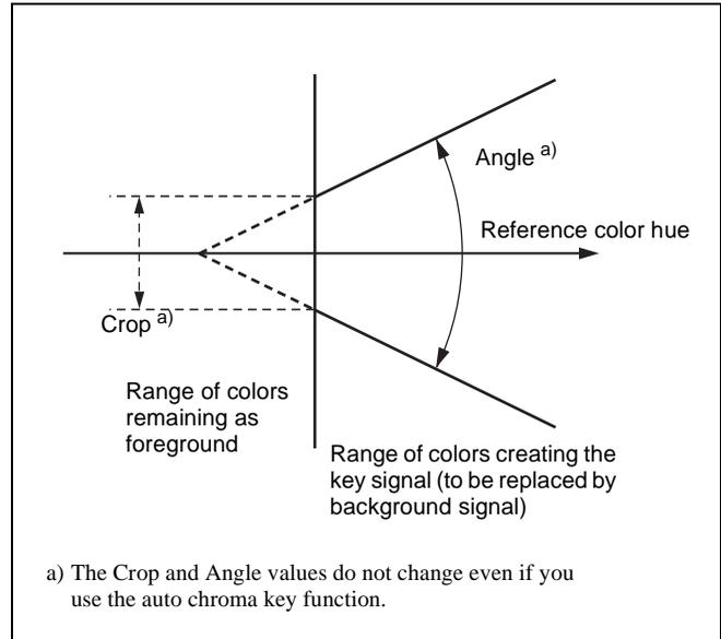
To adjust the window, the Clip, Gain, Hue must be adjusted to appropriate values. Set these to appropriate values first, and then proceed as follows.
