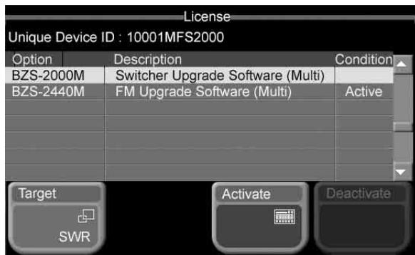
The abbreviation for the currently selected application appears on the [Target] button. The status area shows the device ID (Unique Device ID) for the currently selected application, and the model number, product name, and current state ([Active] or blank) of each of the options available. Unsupported option columns are grayed out.
