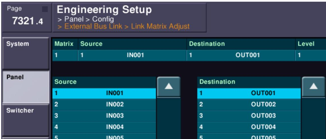
The screenshot shows the 'Engineering Setup' interface for page 7321.4. The breadcrumb trail is '> Panel > Config > External Bus Link > Link Matrix Adjust'. The main table shows Matrix, Source, Destination, and Level. Below the table are two scrollable lists: Source (IN001 to IN005) and Destination (OUT001 to OUT005).
