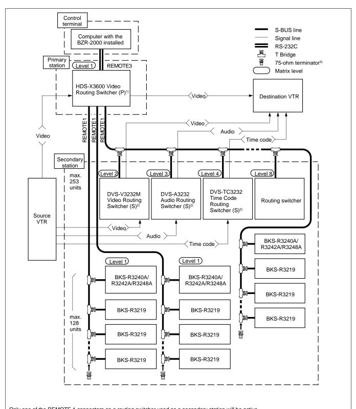
Only one of the REMOTE 1 connectors on a routing switcher used as a secondary station will be active.
