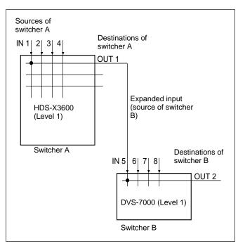
Even when such input expansion is repeated 4 times at maximum, the routing function enables you to search for destinations tracing back via the expanded inputs and obtain a display of the appropriate source.
