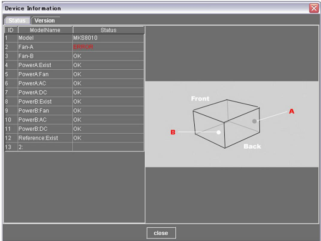
On the MVS-8000, which has a number of cooling fans, an illustration appears, showing the location of the fan, as follows.
