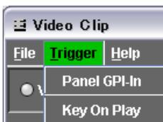
**Panel GPI-In:** Enables clip operations to be carried out via a switch connected to a GPI input port of the SCU (system control unit) controlling the switcher control panel.
