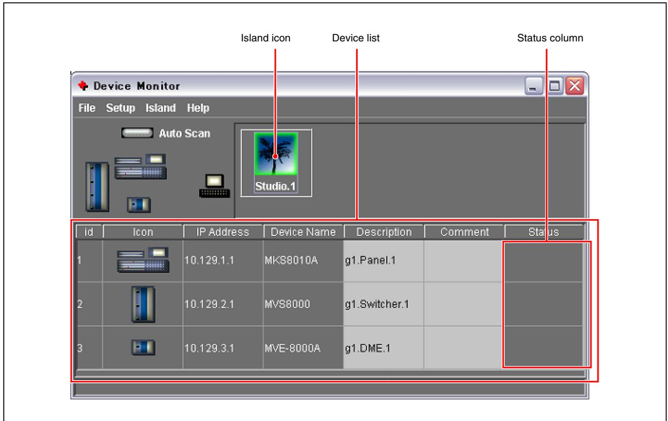
In the example shown above, one of each of a center control panel, switcher processor, and DME processor are present on the network (this combination is termed a “standard configuration”), and these belong to a group called “Studio.1.”
