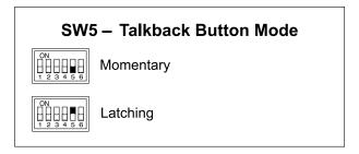
Figure 4. Talkback button mode configuration switch
