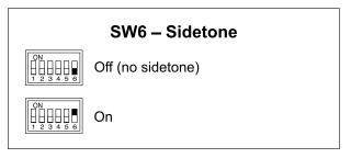
Figure 5. Sidetone function configuration switch
