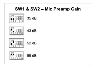
Figure 2. Microphone preamplifier gain configuration switches
