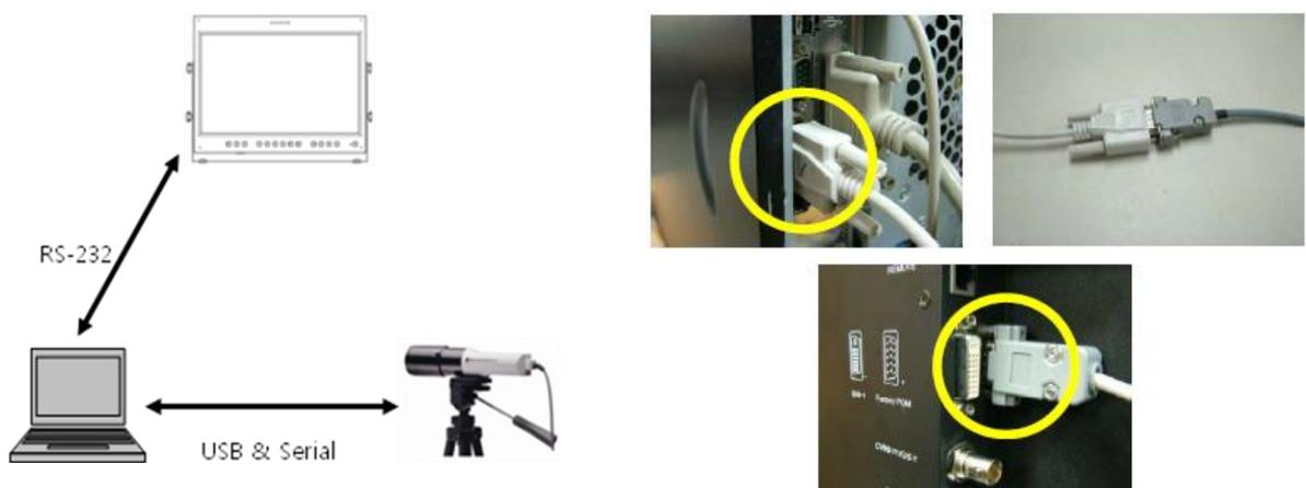
Fig 1: Connecting to the serial port
