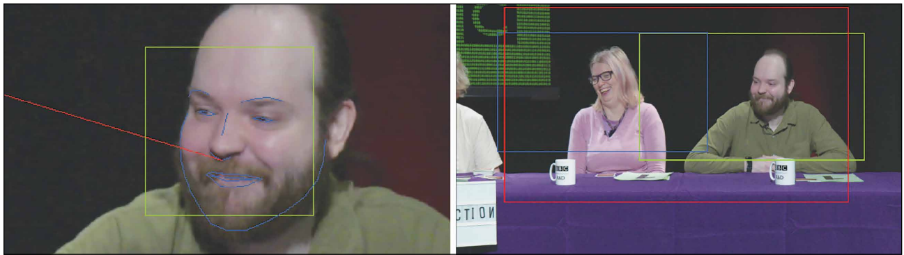
FIGURE 1. The face detection bounding box (green), facial landmarks (blue), and head pose projection (red) (left), and a camera view labelled with three candidate crops: two mid-close shots (green and blue) and a midshot (red) (right).
