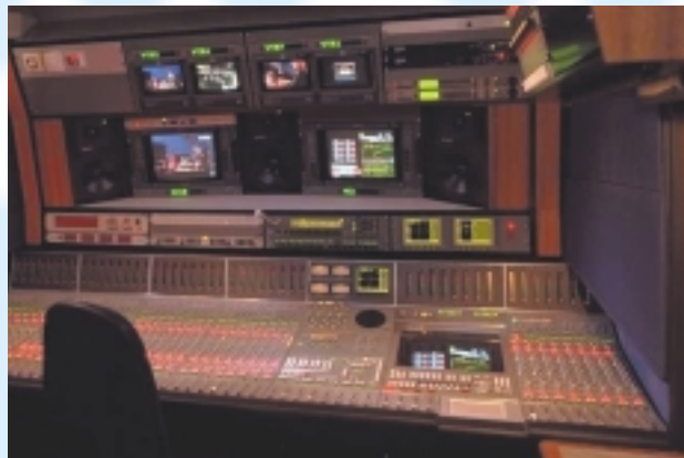
SSL Mixing console and no less than 3 Master Stereo Displays in the large OB-van from TEAM JELBE, Sweden. Photo: Team Jelbe, Sweden
