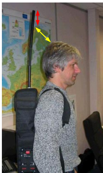
Figure 5 - Rucksack mounted system showing long antenna with radiating section well above the cameraman's head.
