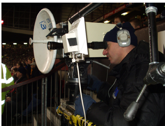
Figure 6 ~ Typical analogue system showing the very directional antenna and telescope used to align it with the transmitter.
