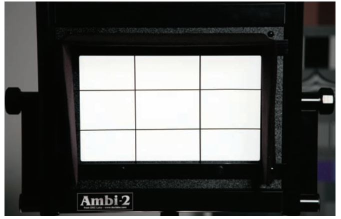
Figure 1b. Ambi Illuminator with grid over transparency.
