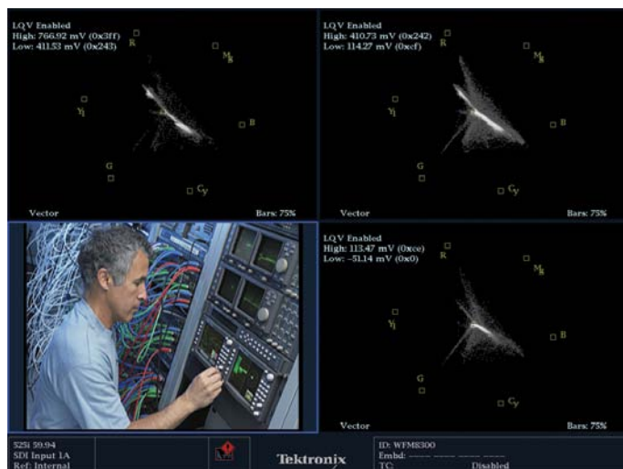
Figure 32. Four-tile display of the WFM 8300 showing multiple vectorscope displays, with independent LQV thresholds.
