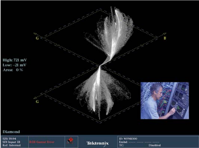
Figure 19. Live signal with blue balance error.
