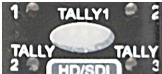
The Tally light can also be activated by the unit’s Auxiliary Output connection. The unit is equipped with three tally lights so that it can display GPI information in different colors for different members of the crew or talent, when required. These lights light up red green and yellow.
