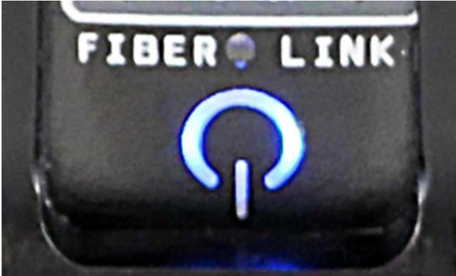
Below that is the power button for the entire camera I/O (TX) unit. This light should be lit at all times when the unit is in use. Push this button once to power on the unit. Hold the button for two or three seconds to power off (this is a security feature). MultiDyne offers a special version of the SilverBack Camera I/O unit that is always powered on.
