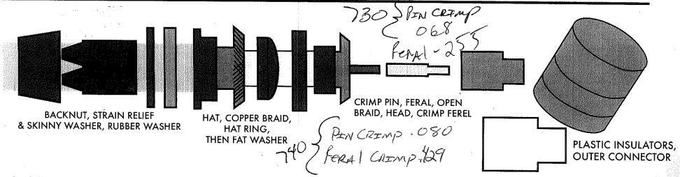
1.) Slide on the backnut, strain relief, skinny washer, and rubber washer (with groove facing end on 740 cable).
