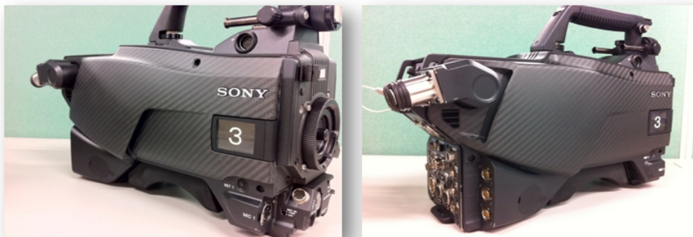
Picture 11 shows the carbon graphite side cover of HDC-2500-series
