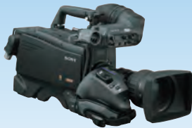
HDC-1500R Optical-fiber interface 1080/50i, 59.94i 1080/23.98P, 24P, 25P, 29.97P 1080/50P*, 59.94P* 720/50P, 59.94P
