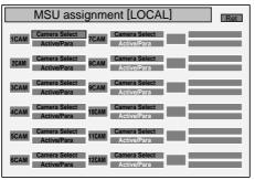
6. Select the control functions for each camera. Camera Select: Selection by the corresponding camera select button on the MSU-700A/750 Active/Para: Control from the MSU-700A/750 in Panel Active/Parallel mode.
