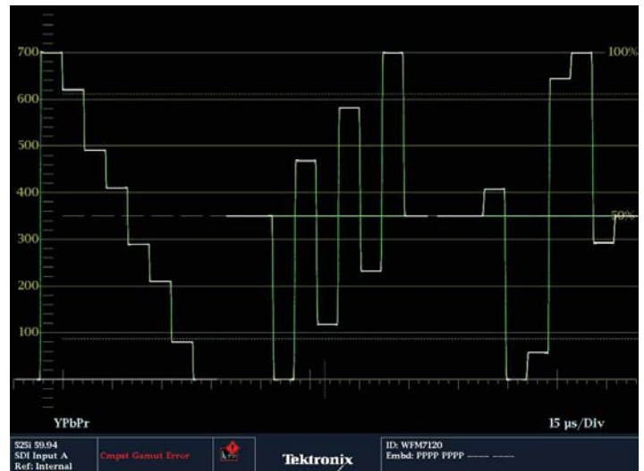
Figure 98. WFM7120 Y/C'b/C'r display of 100% color bars.
