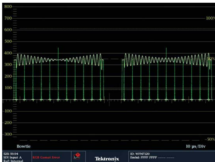
Figure 94. Y & Pb Left and Y & Pr right.
