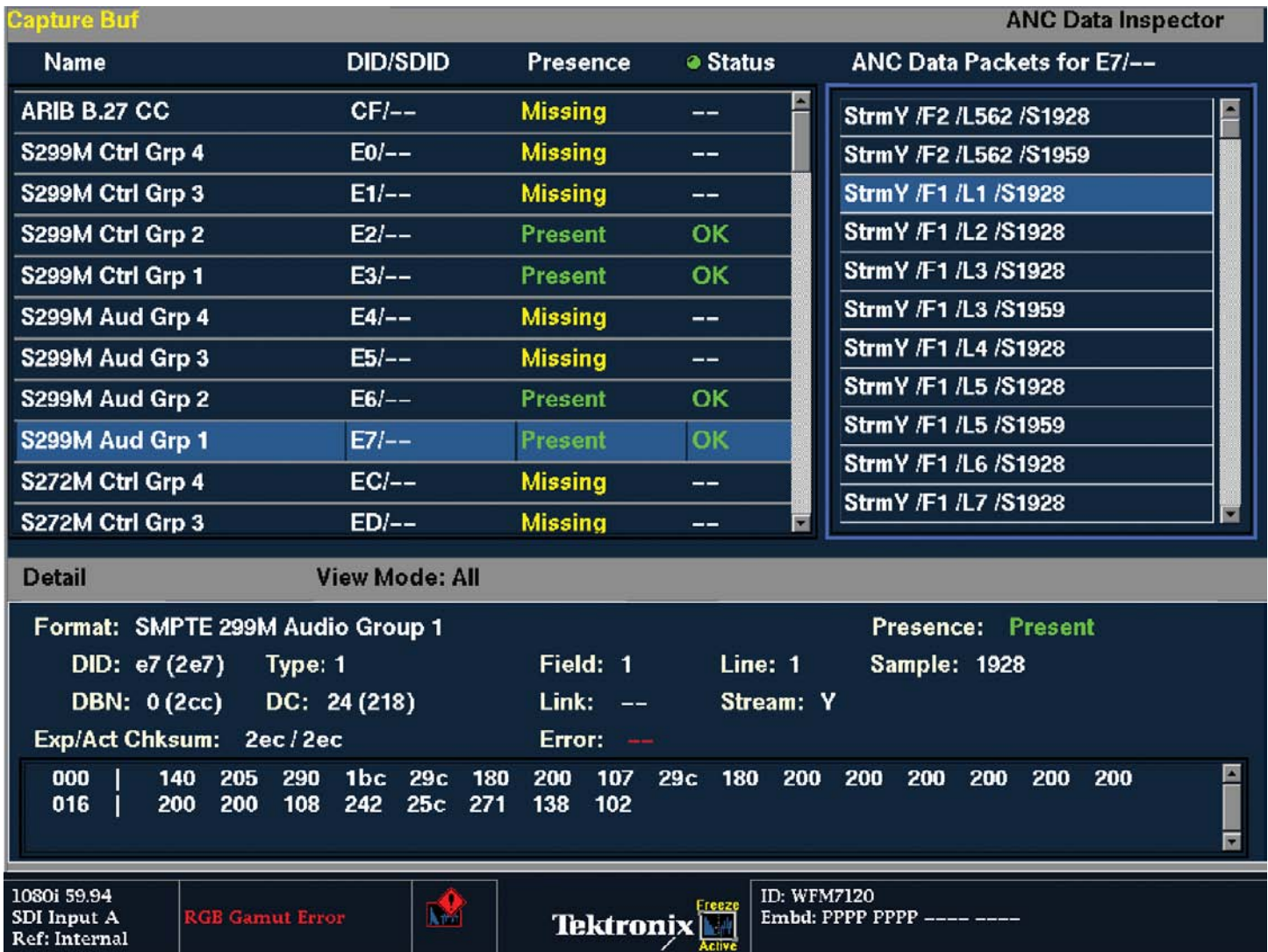
Figure 66. Capture Buffer display using Ancillary Data Inspector.
