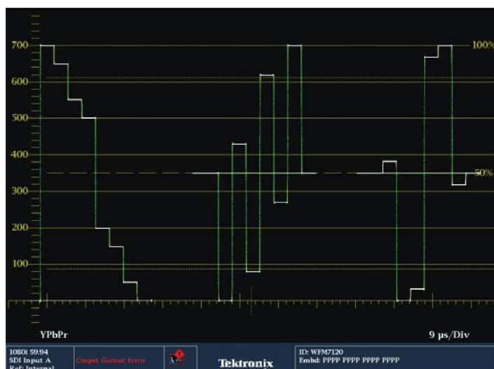
Figure 111. 100% color bar signal YPbPr for HD.
