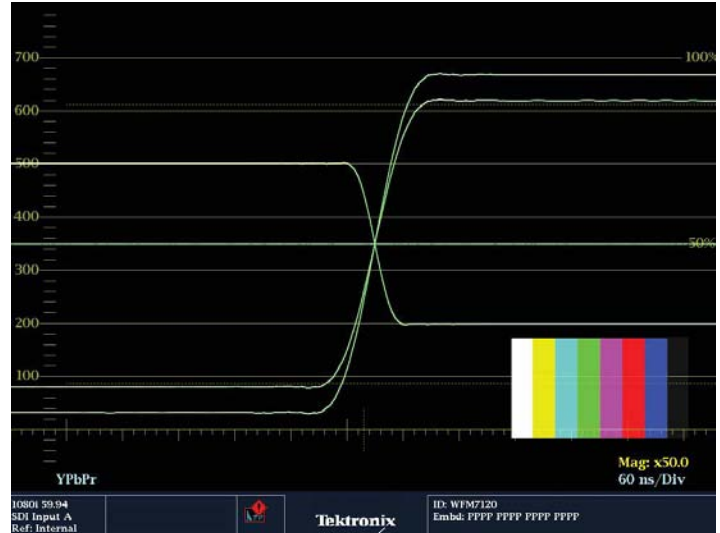
Figure 90. Interchannel timing measurement using green/magenta transition.
