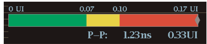
Figure 87. Jitter Bar Measurement.
