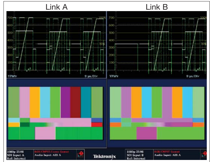
Figure 36. Waveform displays of Dual Link A and B signal for R'G'B' (A) 4:4:4:4 format.
