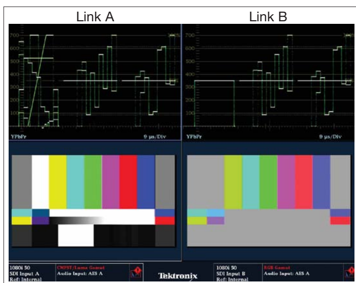
Figure 37. Waveform displays of Dual Link A and B signals for Y'C'bC'r (A) 4:4:4:4 10-bit format.
