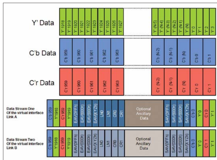
Figure 48. Level B mapping structure for Dual Link fast progressive signals in a 3 Gb/s interface.
