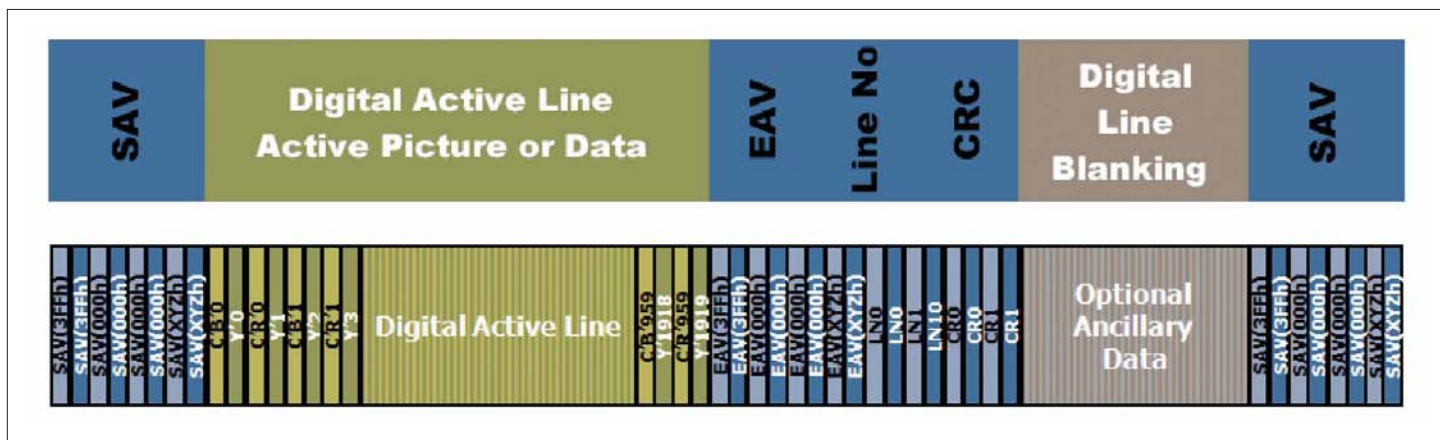
Figure 34. SDI data structure for a single line.
