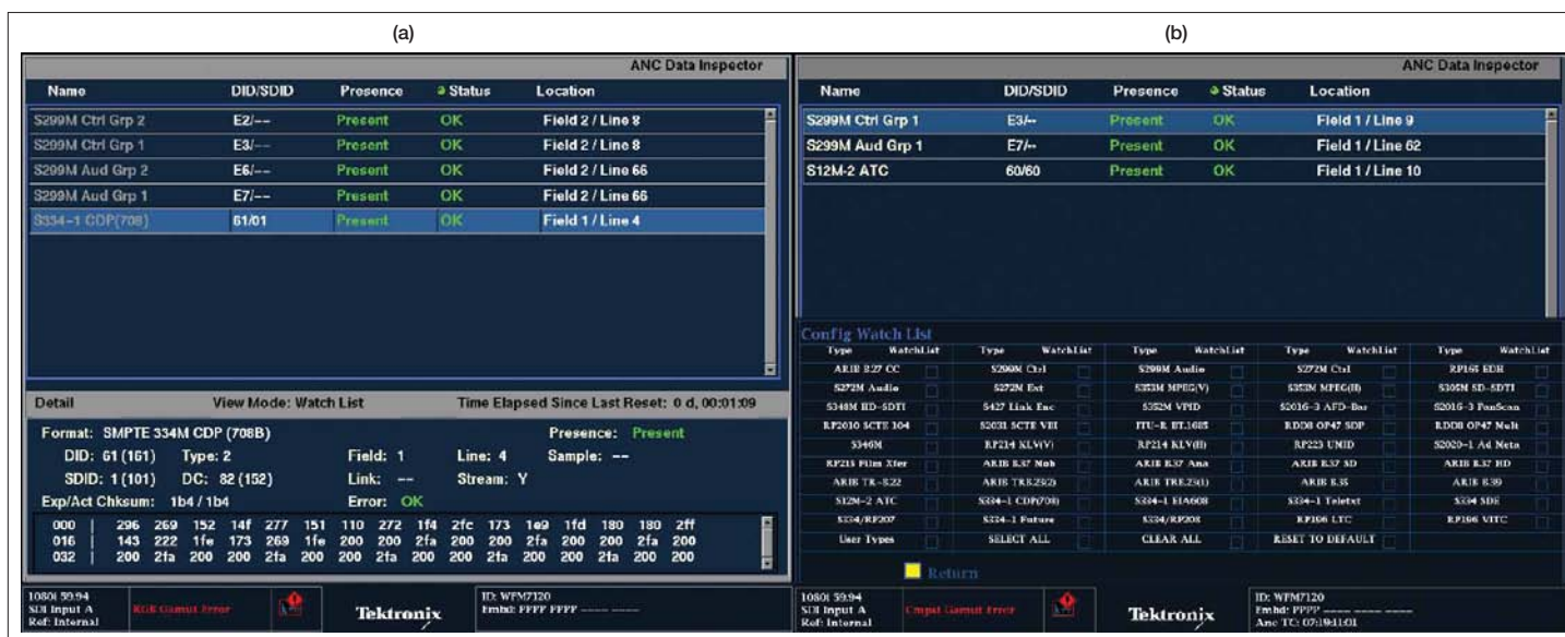
Figure 65. Ancillary data on the WFM7120: (a) ANC Data Inspector; (b) Watch List configuration.
