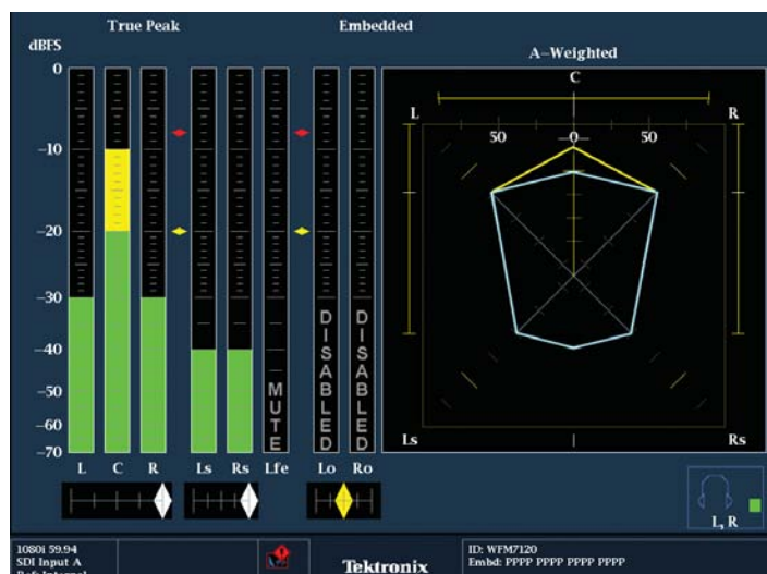
Figure 62. Surround Sound Display with live audio signal.
