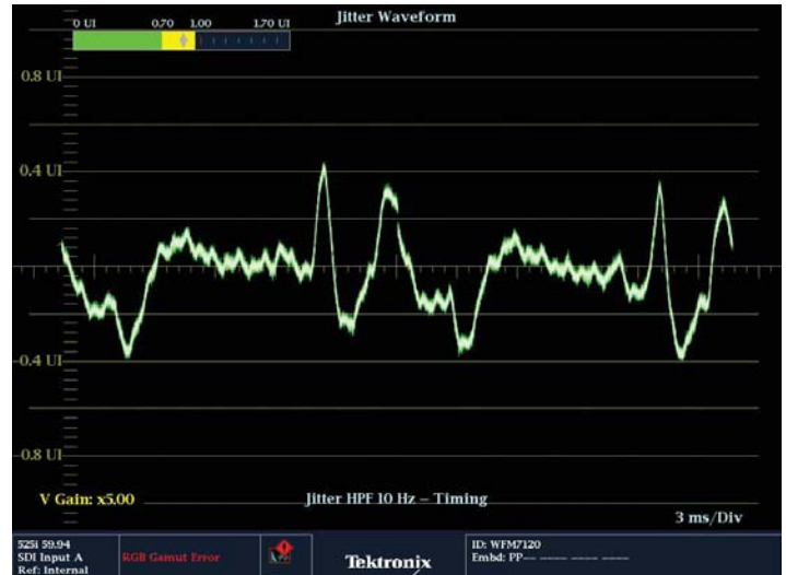
Figure 86. Jitter display mode in two-field sweep on WFM7120.
