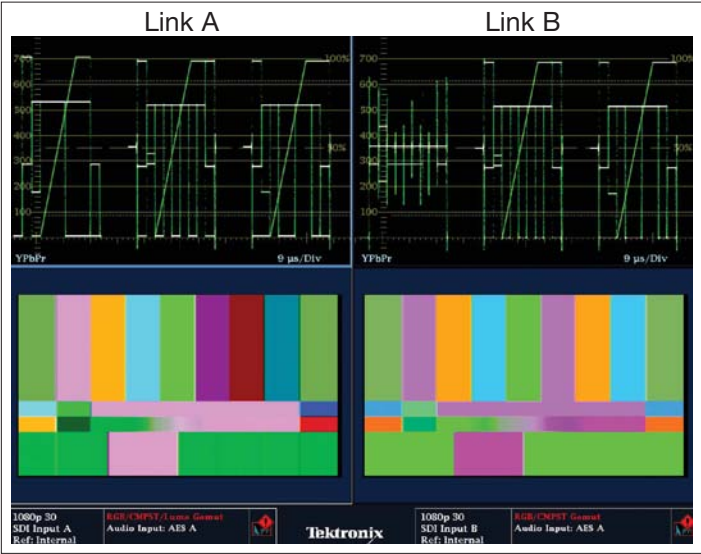
Figure 39. Waveform displays of Dual Link A and B signals for R'G'B' 4:4:4 12-bit format.
