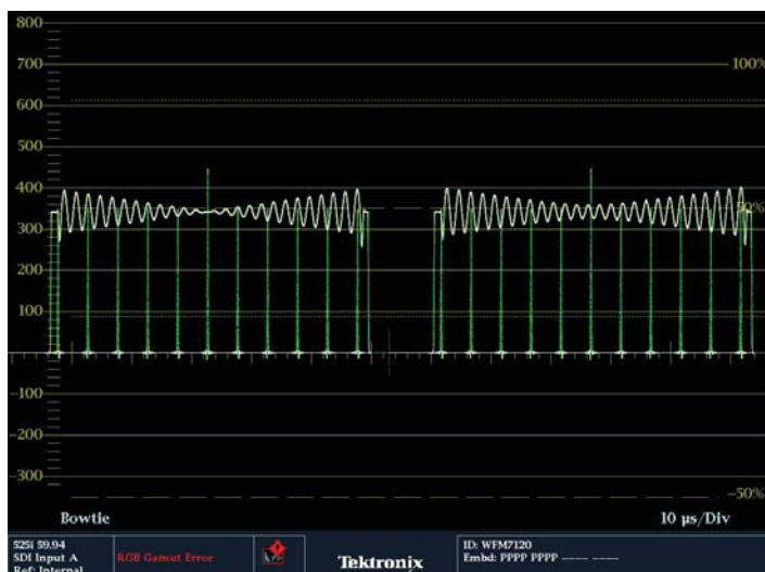
Figure 96. Bowtie display Pr gain error vs. Y.
