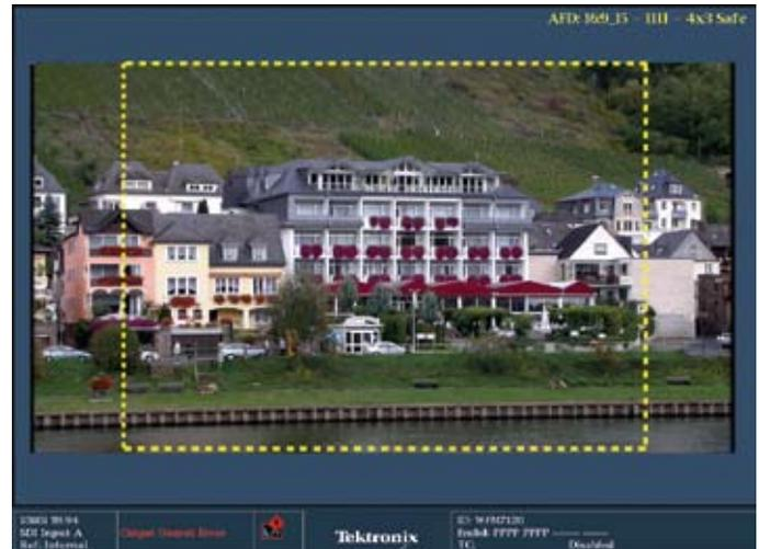
Figure 8. Picture display showing Active Format Descriptor information.
