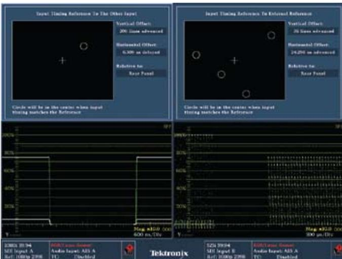
Figure 16. Simultaneous Timing Displays of HD and SD.
