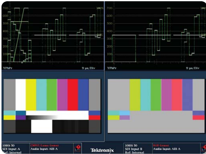
► Figure 4. Waveform displays of Dual Link A and B signals for Y'C'bC'r(A) 4:4:4:4 10-bit format.
