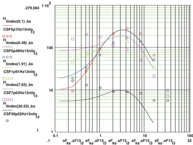
► **Figure 6.** An example of model (solid) vs. human vision response (points) (31): Pedestal Luminance is 13 nits. Horizontal: spatial frequency, vertical: contrast sensitivity, curves: temporal frequencies.
