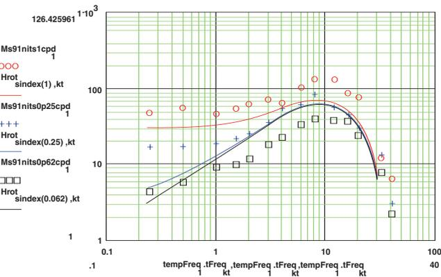
► **Figure 7.** The same as Figure 6 except for 91 nits (45) and the temporal frequency varies along the horizontal while each curve represents a different spatial frequency.
