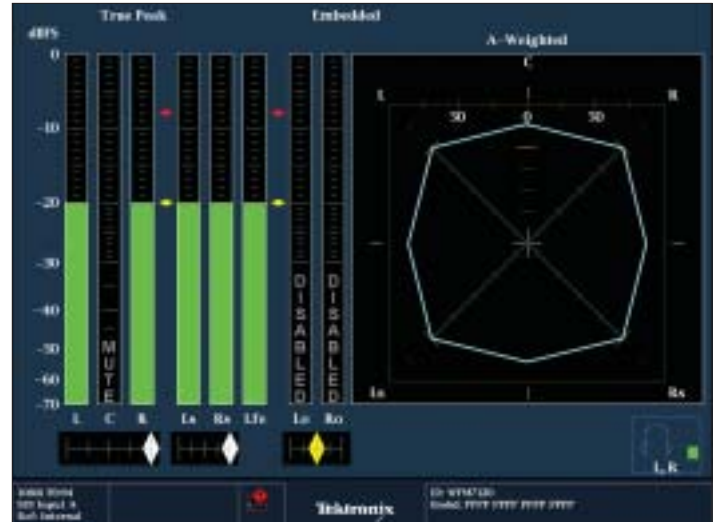
Figure 61. Surround Sound Display with test tones for L, R, Ls and Rs.
