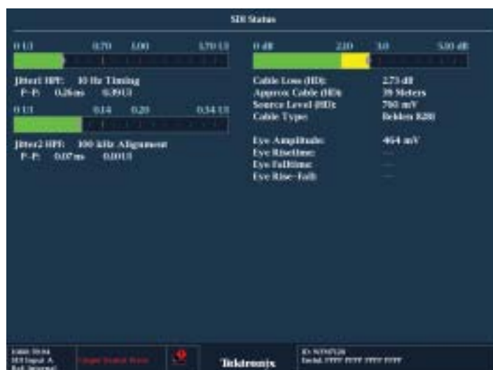
Figure 89. SDI Status display from WFM7120.
