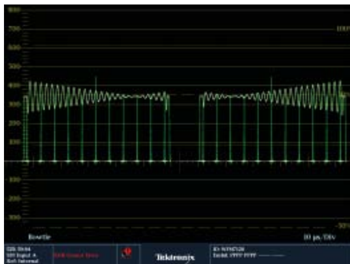
Figure 95. Bowtie display, Pb delayed 55ns, Pr advanced 50ns Y.
