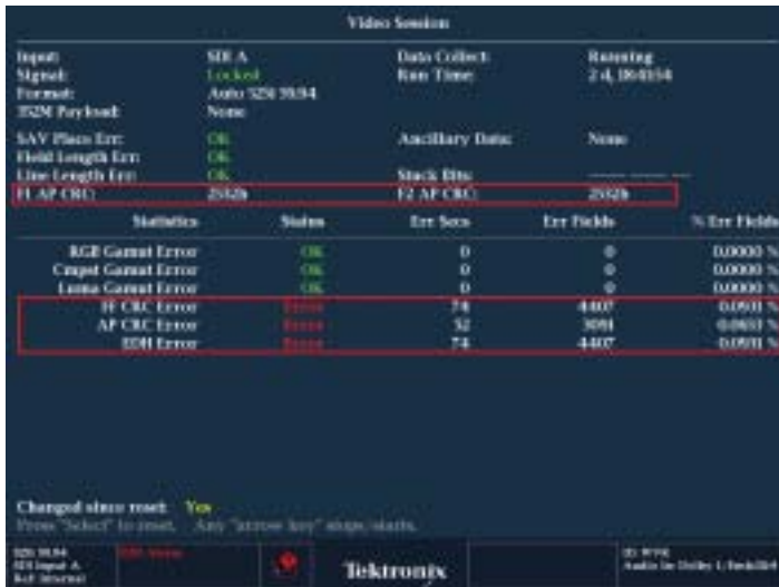
Figure 79. Video Session screen of SD signal showing EDH values on WVR7120.
