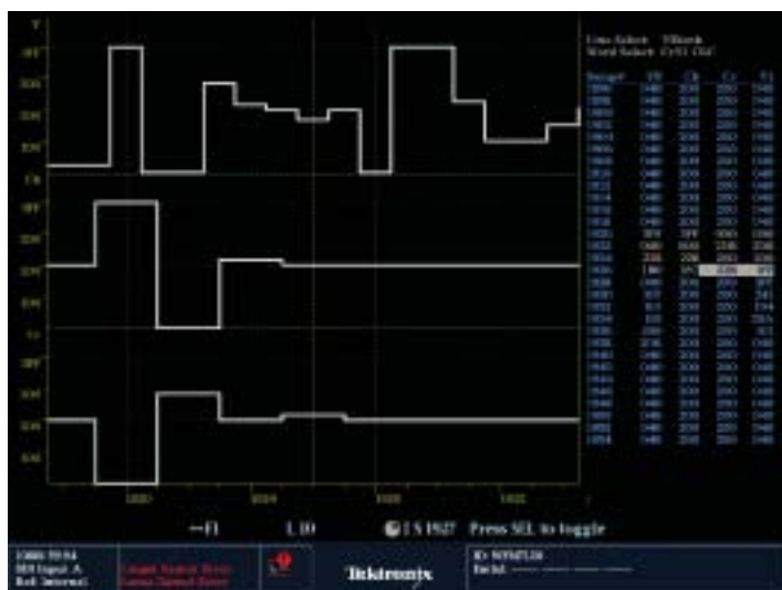
Figure 64. Data list display of the WFM7120 showing the ancillary data of a SMPTE352M packet.
