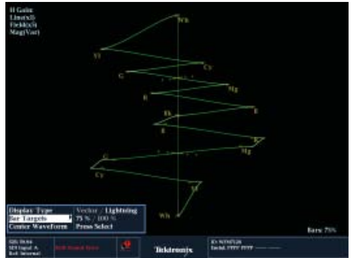
Figure 104. Lightning display with P'r gain error.
