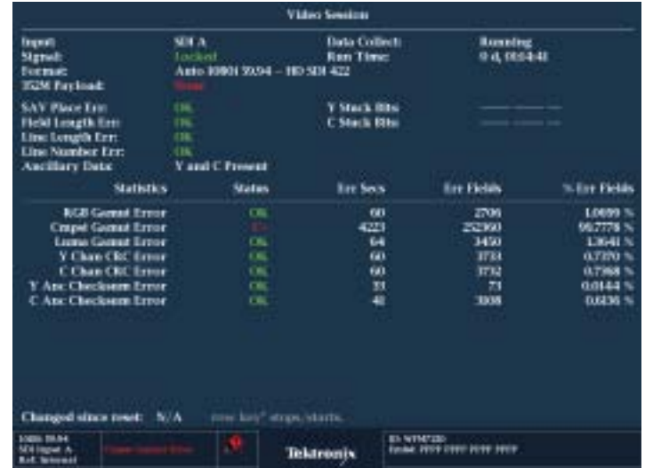
Figure 80. Video Session screen of HD signal showing CRC values on WFM7120.
