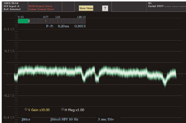
Jitter display with 10Hz filter
