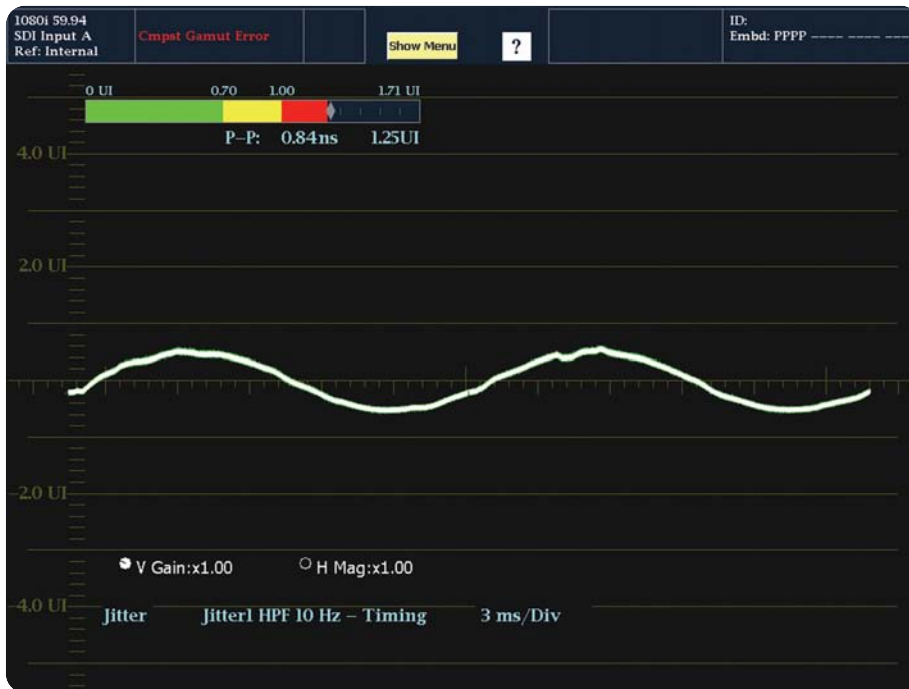
► Figure 12. 60Hz mains frequency jitter.
