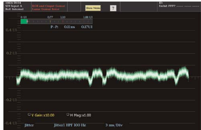
Jitter display with 100Hz filter
