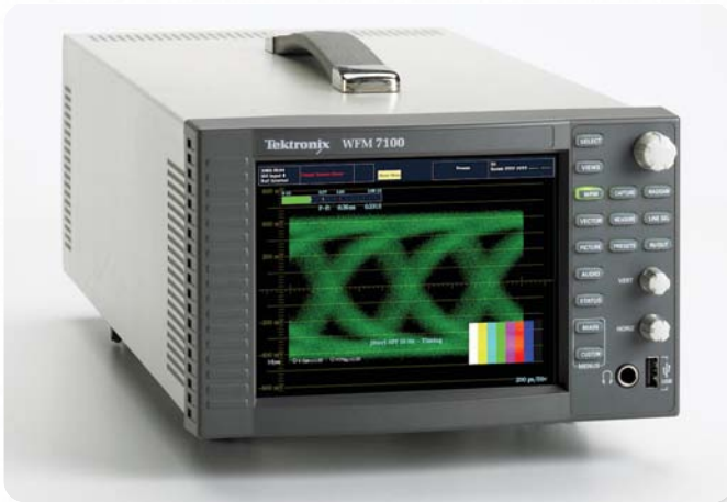
► Figure 3. WFM7100 waveform monitor showing eye display.
