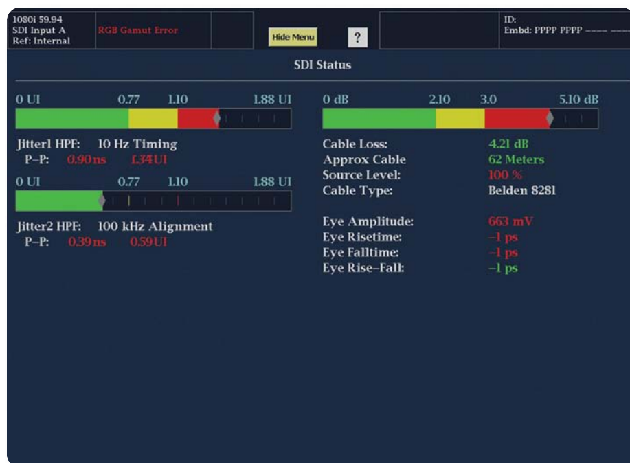
► Figure 21. SDI status display showing cable length measurement.
