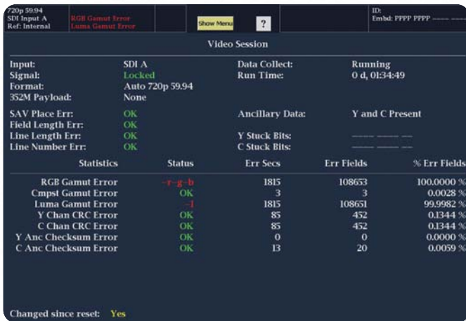
► Figure 2. Status display showing CRC errors of an HD SDI signal.
