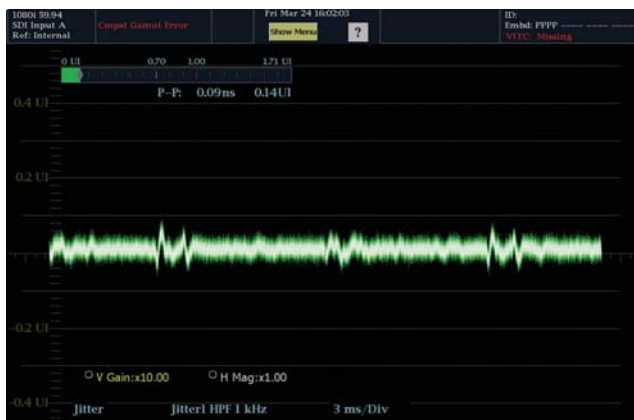
Jitter display with 1 kHz filter
