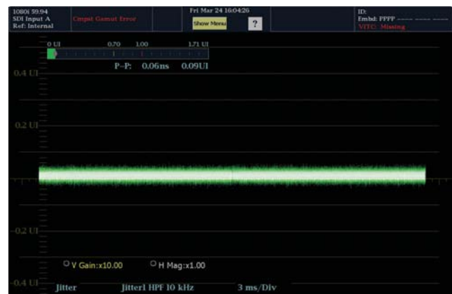
Jitter display with 100 kHz filter
