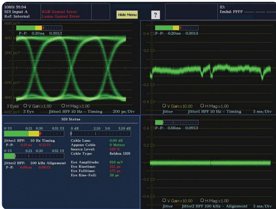
► Figure 13. Simultaneous measurement of timing and alignment jitter.
